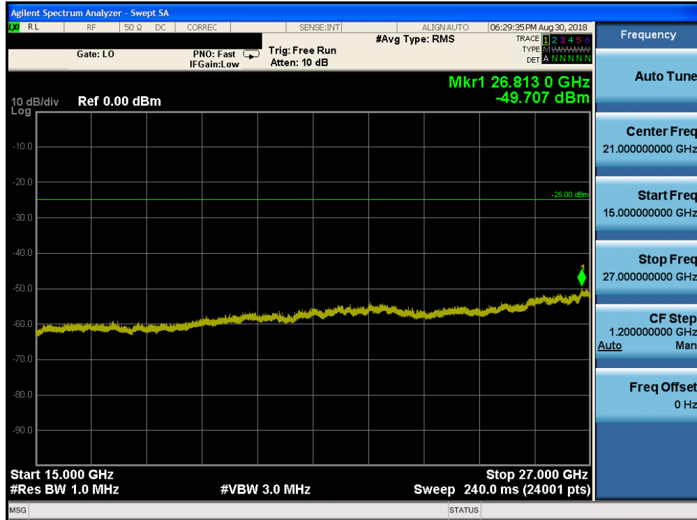
Plot 7-156. Conducted Spurious Plot (Band 41 – 20.0MHz QPSK – RB Size 1, RB Offset 0 – Low Channel)
