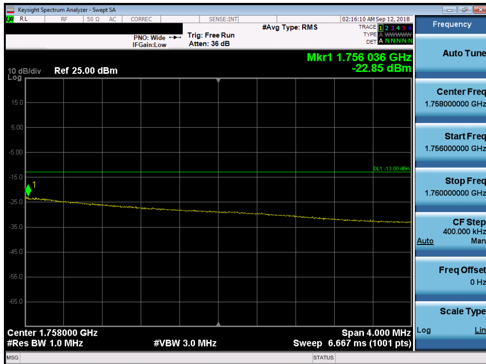
Plot 7-218. Upper Extended Band Edge Plot (Band 4 – 15.0MHz QPSK – RB Size 75)
