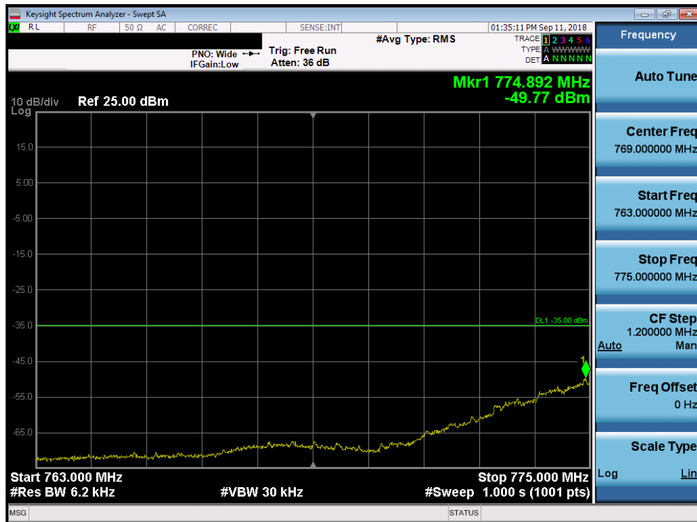
Plot 7-180. Lower Emission Mask Edge Plot (Band 13 – 10.0MHz QPSK – RB Size 50)
