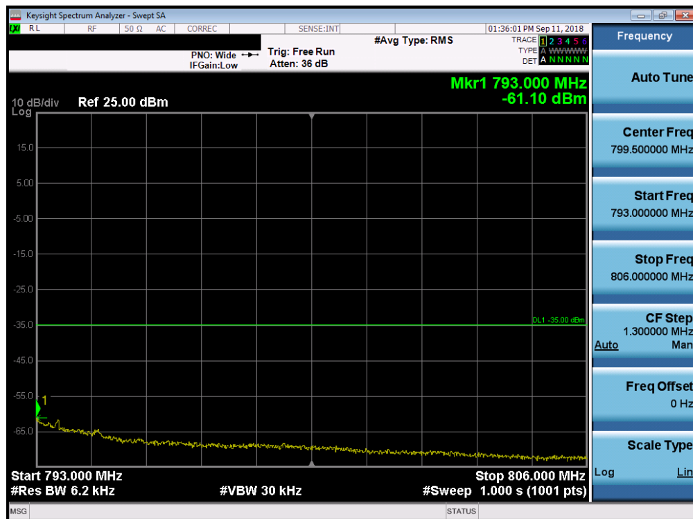
Plot 7-182. Upper Emission Mask Edge Plot (Band 13 – 10.0MHz QPSK – RB Size 50)
