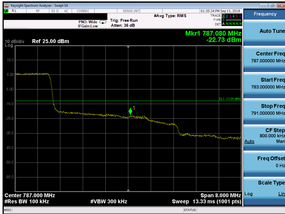
Plot 7-181. Upper Band Edge Plot (Band 13 – 10.0MHz QPSK – RB Size 50)
