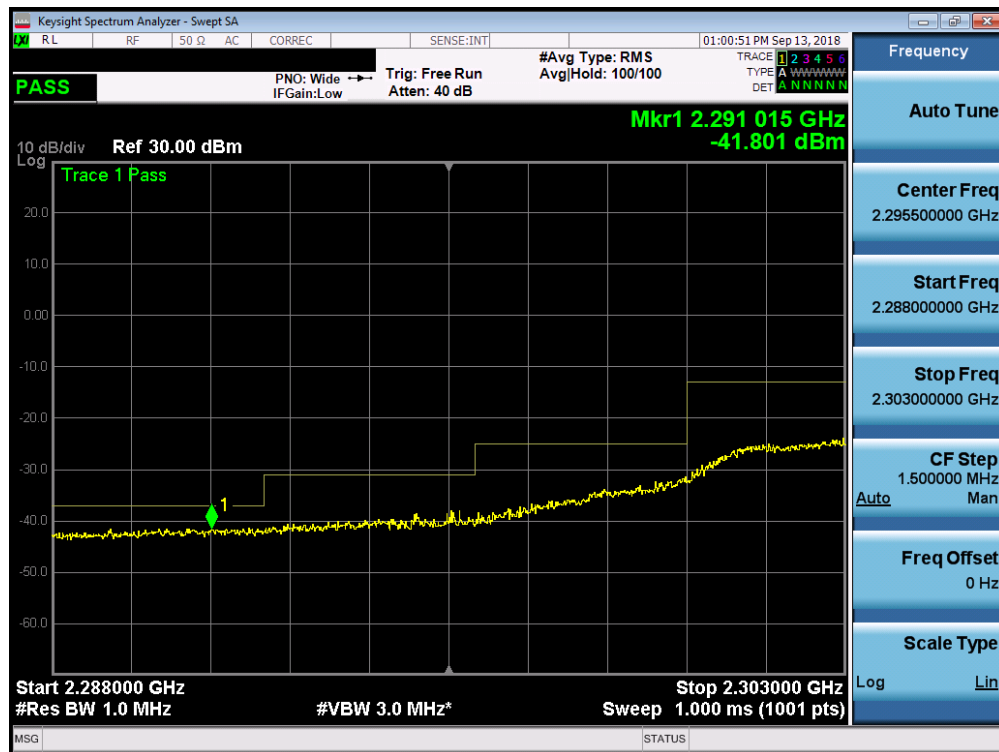
Plot 7-296. Lower Extended Band Edge Plot 2288 MHz – 2303 MHz (Band 30 – 5.0MHz QPSK – RB Size 25)
