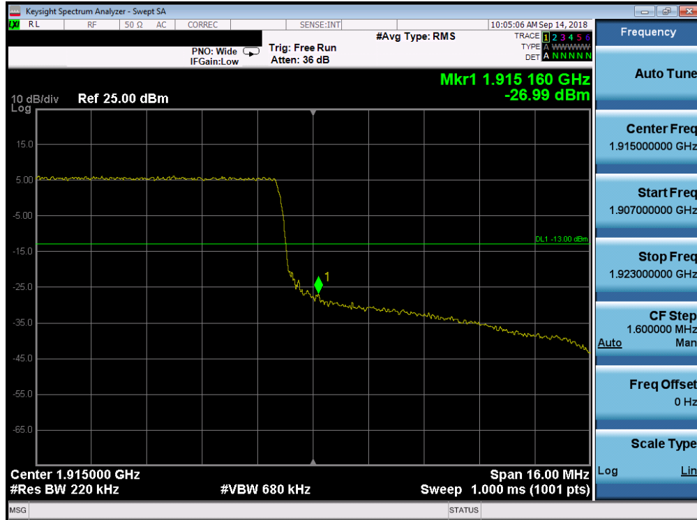
Plot 7-293. Upper Band Edge Plot (Band 25 – 20.0MHz QPSK – RB Size 100)
