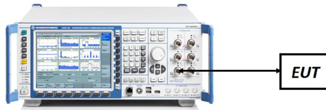
Figure 7-4. Conducted Power Measurement Setup
