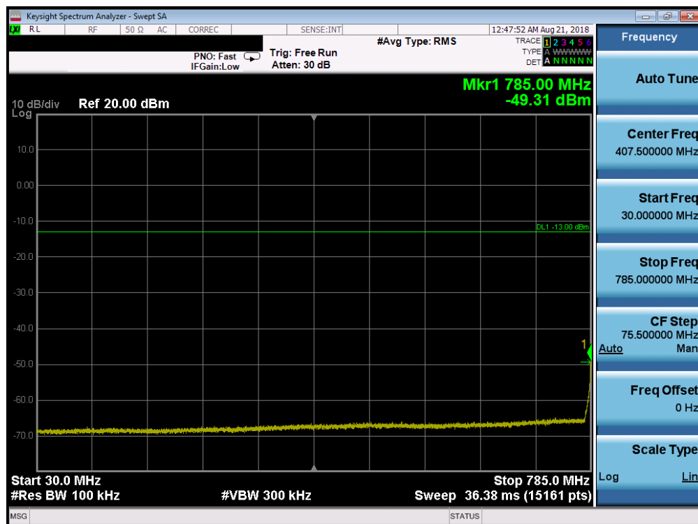
Plot 7-28. Conducted Spurious Plot (LTE Band 14, 5 MHz QPSK – RB Size 1, RB Offset 0 – Mid Channel)
