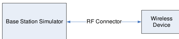
Figure 8-2 Power Measurement Setup
