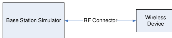
Figure 8-3 Power Measurement Setup
