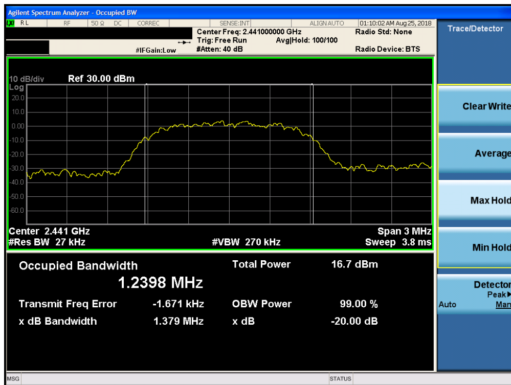
Plot 7-17. 20dB Bandwidth Plot ANT 2 (Bluetooth, 8DPSK, ePA – Ch. 39)
