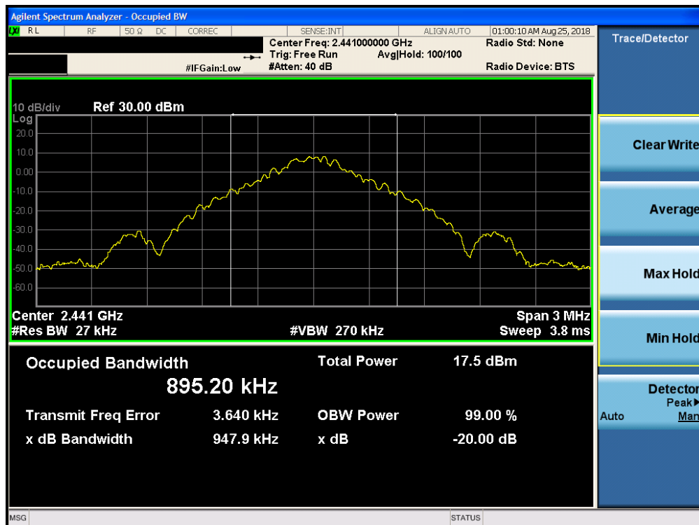
Plot 7-14. 20dB Bandwidth Plot ANT 2 (Bluetooth, GFSK, ePA – Ch. 39)
