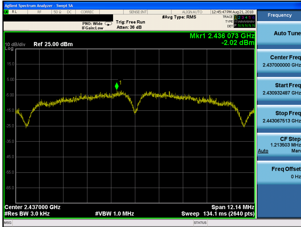
Plot 7-29. Power Spectral Density Plot SISO Core 0 (802.11b – Ch. 6)
