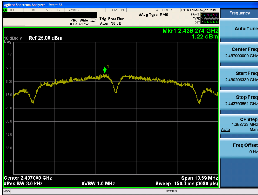
Plot 7-47. Power Spectral Density Plot SISO Core 1 Diversity (802.11b – Ch. 6)
