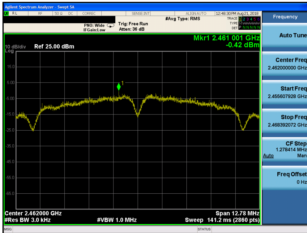
Plot 7-30. Power Spectral Density Plot SISO Core 0 (802.11b – Ch. 11)
