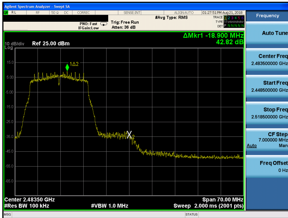
Plot 7-88. Band Edge Plot SISO Core 0 (802.11n (2.4GHz) – Ch. 11)
