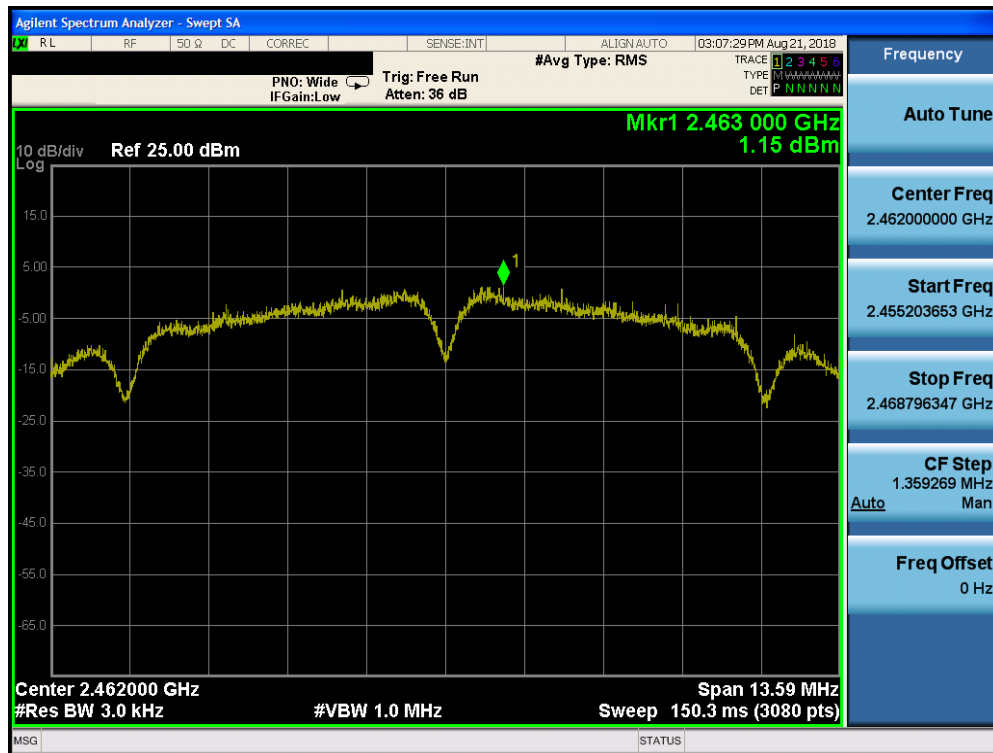
Plot 7-48. Power Spectral Density Plot SISO Core 1 Diversity (802.11b – Ch. 11)
