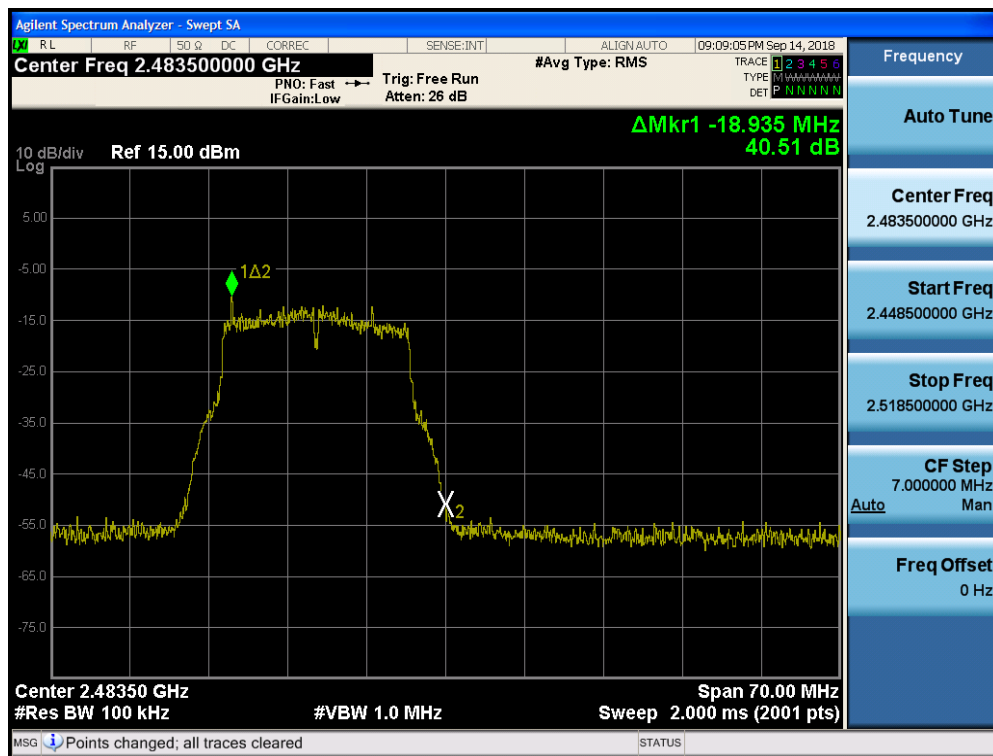
Plot 7-86. Band Edge Plot SISO Core 0 (802.11g – Ch. 13)
