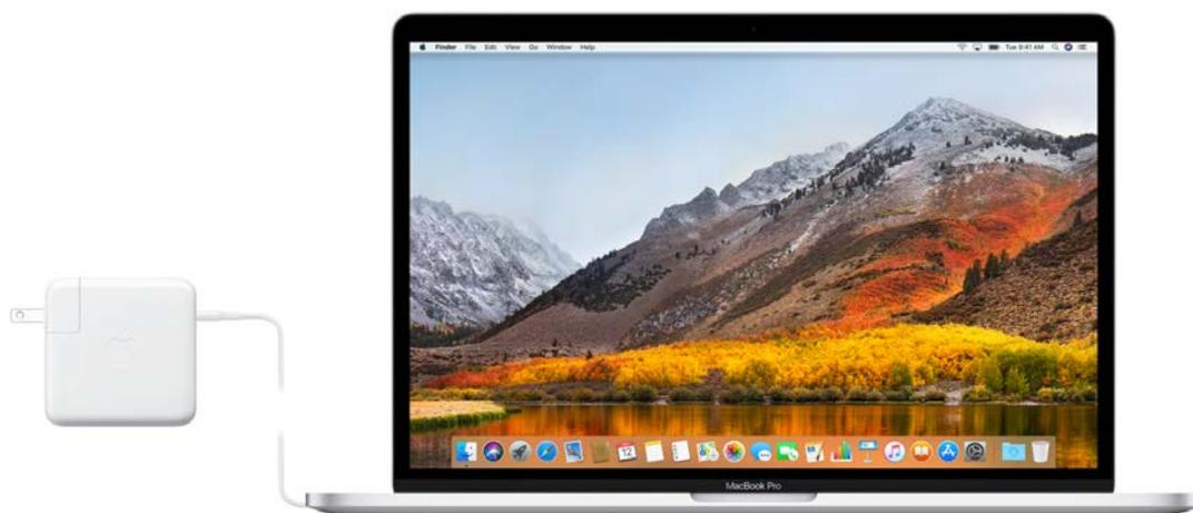
**Charge the battery.** Connect your MacBook Pro to a power outlet using the included USB-C Charge Cable and 61W or 87W USB-C Power Adapter.
