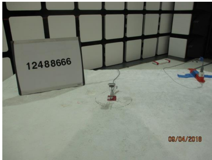
RADIATED EMISSIONS ABOVE 30 MHz (Back – With Watch)
