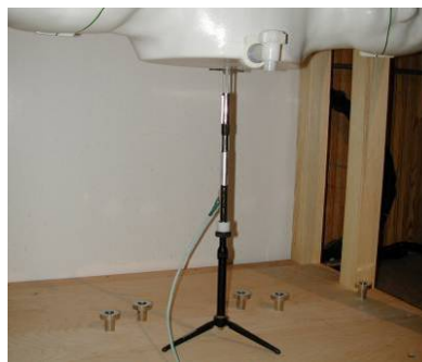
Figure 9-2 System Verification Setup Photo
