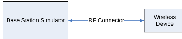
Figure 8-2 Power Measurement Setup
