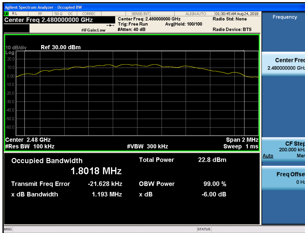
Plot 7-18. 6dB Bandwidth Plot ANT2 (Bluetooth (LE), 2Mbps, ePA – Ch. 39)
