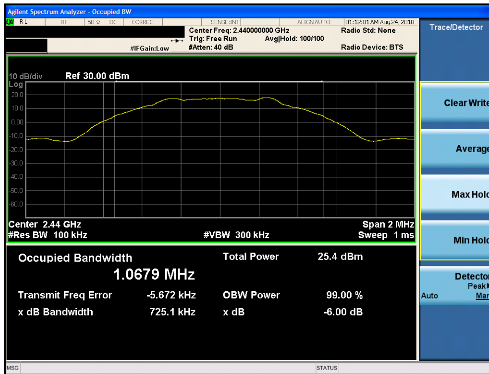
Plot 7-14. 6dB Bandwidth Plot ANT2 (Bluetooth (LE), 1Mbps, ePA – Ch. 19)
