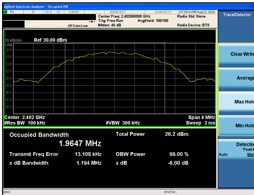
Plot 7-4. 6dB Bandwidth Plot ANT0 (Bluetooth (LE), 2Mbps, ePA – Ch. 0)
