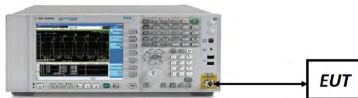
Figure 7-3. Test Instrument & Measurement Setup
