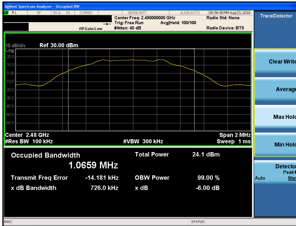
Plot 7-3. 6dB Bandwidth Plot ANT0 (Bluetooth (LE), 1Mbps, ePA – Ch. 39)
