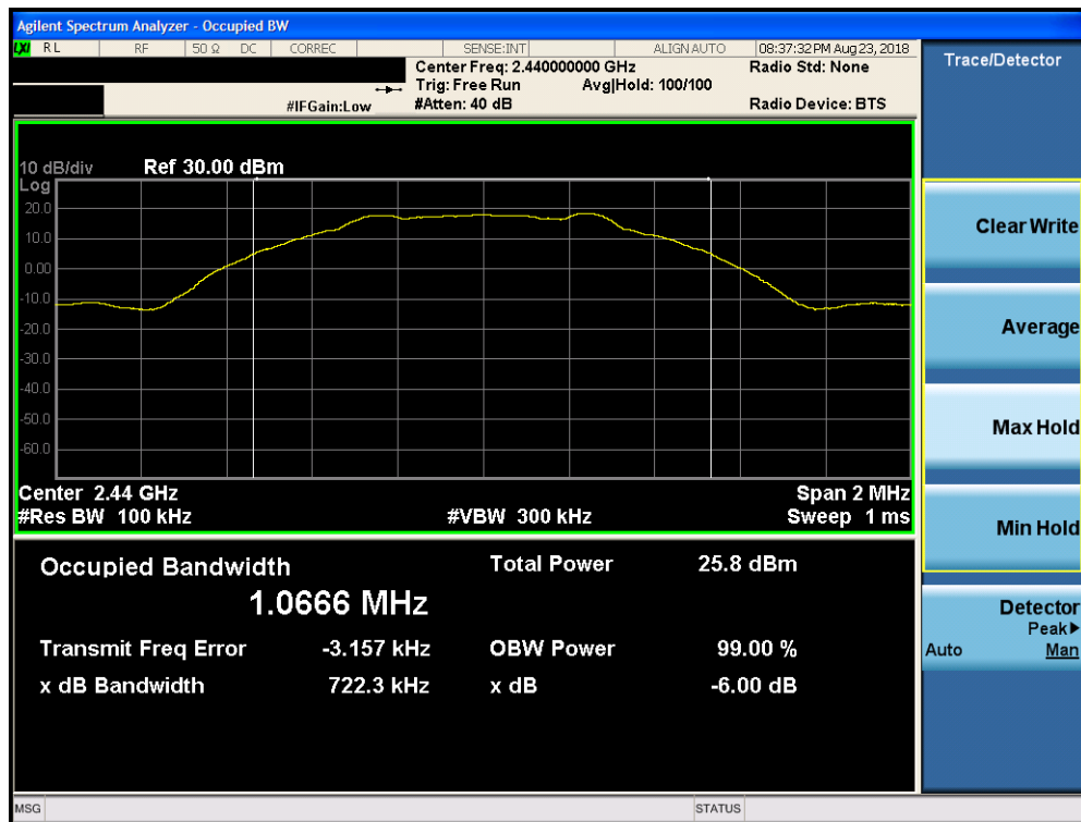
Plot 7-8. 6dB Bandwidth Plot ANT1 (Bluetooth (LE), 1Mbps, ePA – Ch. 19)
