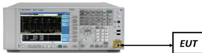
Figure 7-3. Test Instrument & Measurement Setup
