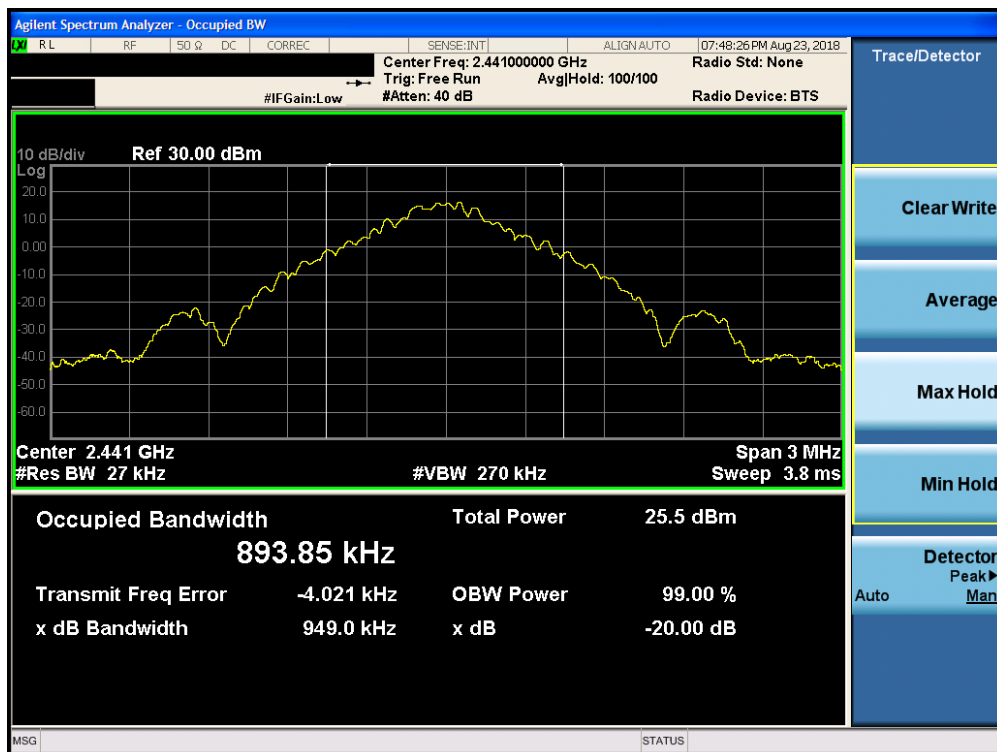
Plot 7-8. 20dB Bandwidth Plot ANT 1 (Bluetooth, GFSK, ePA – Ch. 39)
