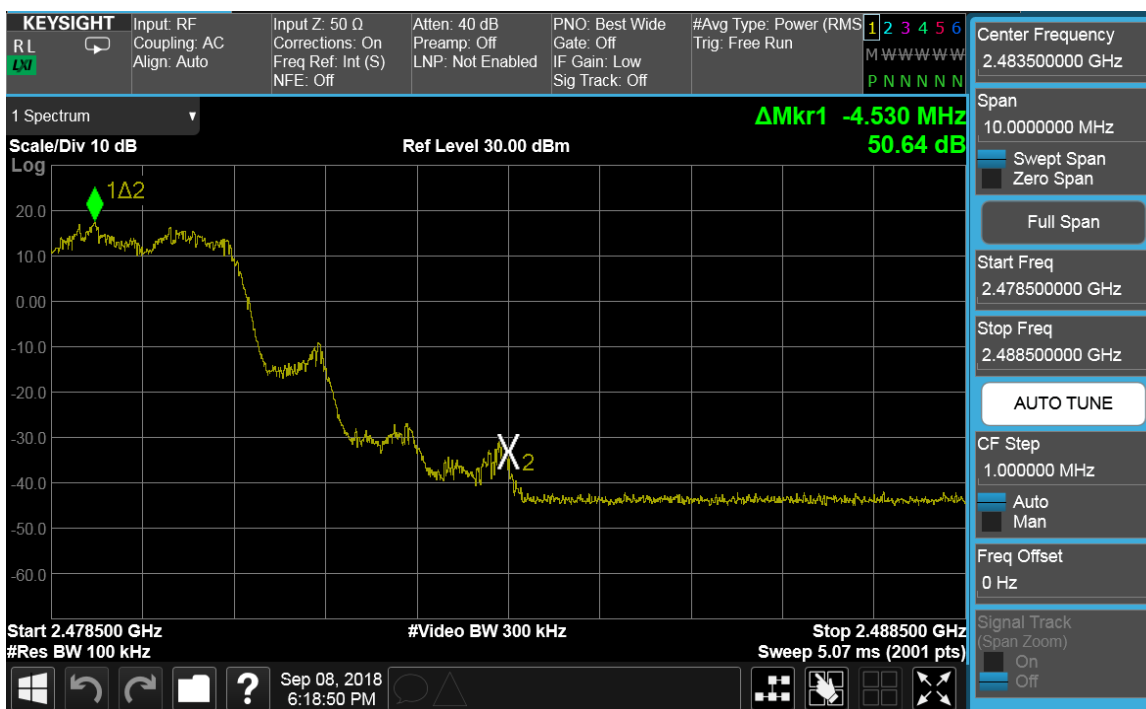
Plot 7-34. Band Edge Plot ANT 1 (Bluetooth with Hopping Enabled, 8DPSK, ePA)
