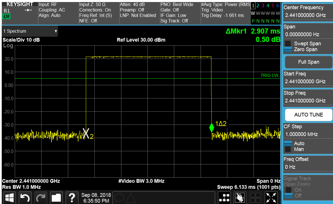
Plot 7-50. Time of Occupancy Plot ANT0(Bluetooth, 8DPSK, ePA)
