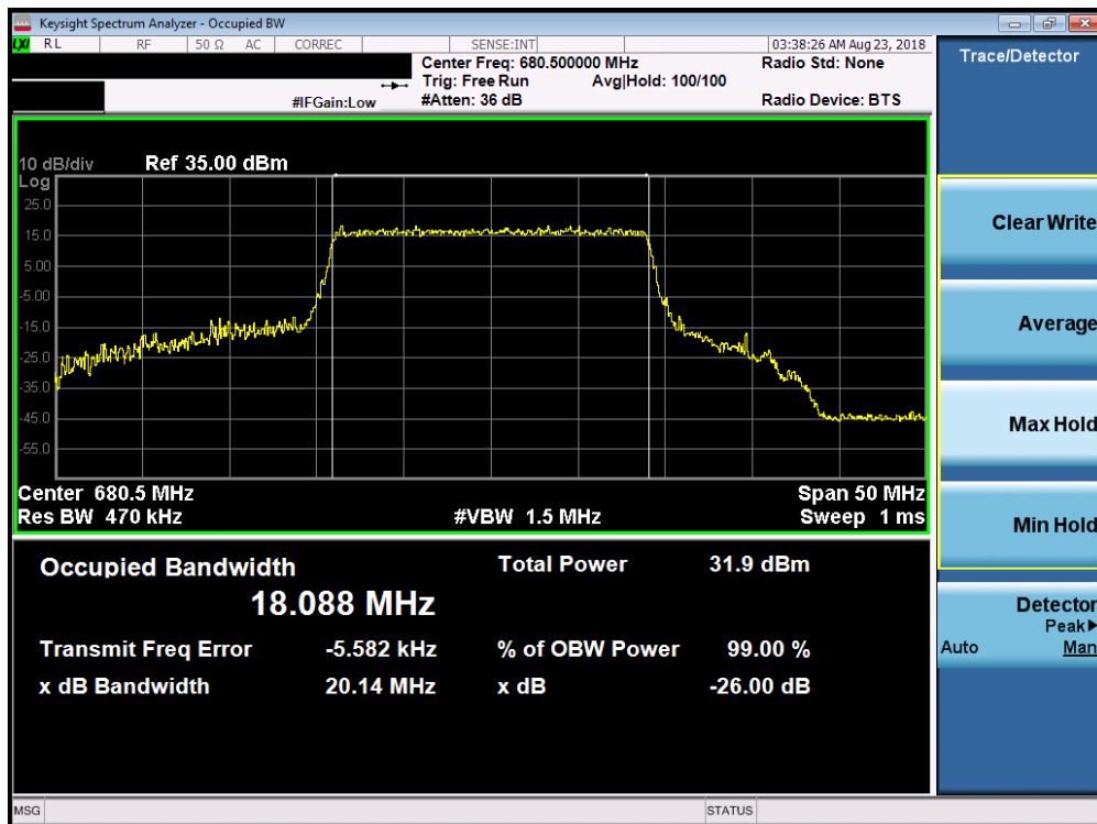
Plot 7-12. Occupied Bandwidth Plot (Band 71 – 20.0MHz 64-QAM – RB Size 100)
