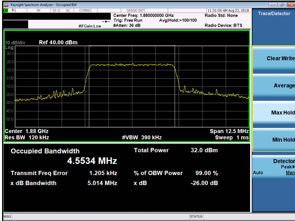
Plot 7-69. Occupied Bandwidth Plot (Band 25/2 – 5.0MHz 64-QAM – RB Size 25)
