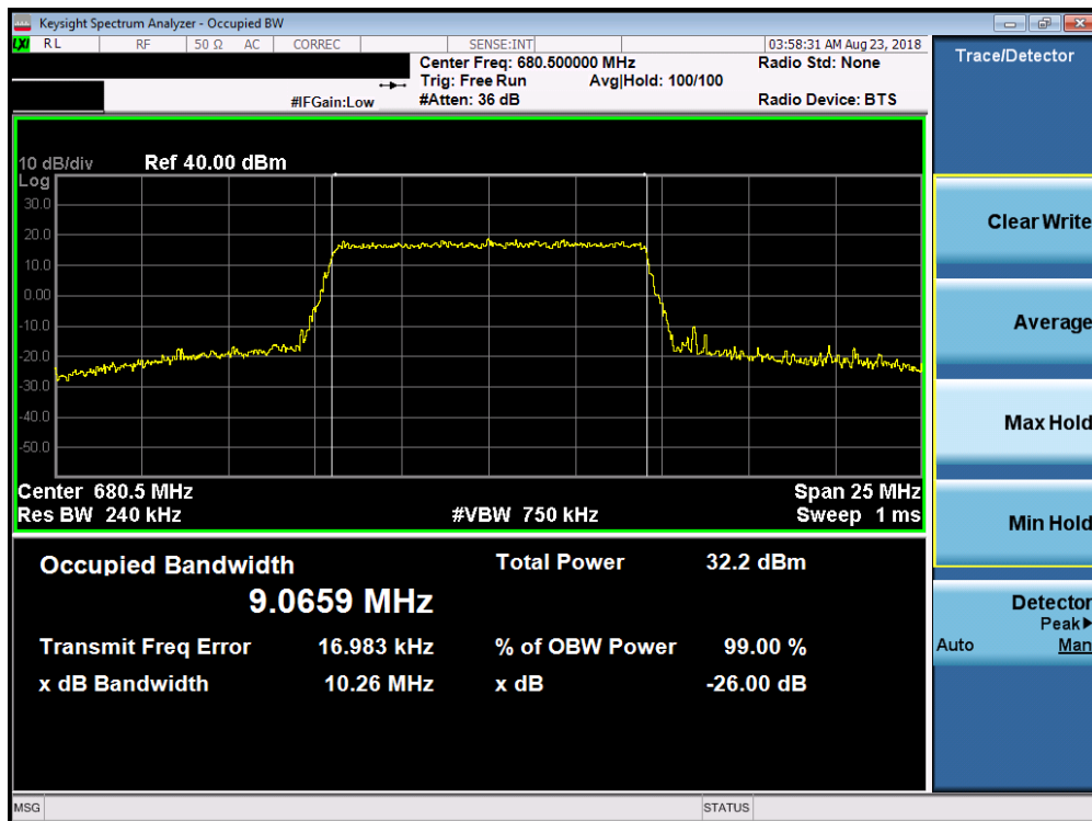
Plot 7-6. Occupied Bandwidth Plot (Band 71 – 10.0MHz 64-QAM – RB Size 50)
