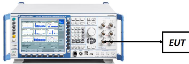
Figure 7-4. Conducted Power Measurement Setup
