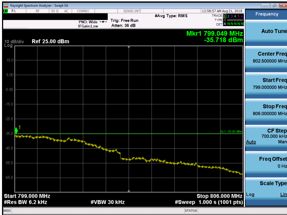
Plot 7-44. Upper Emission Mask Plot (LTE Band 14, 5MHz QPSK – RB Size 25)
