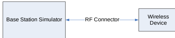
Figure 8-2 Power Measurement Setup
