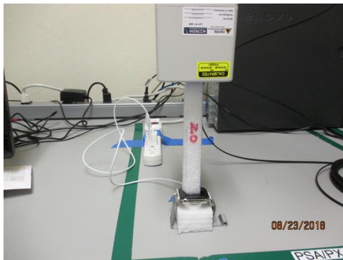
CENTER, RF EXPOSURE SETUP PHOTO (HORIZONTAL) 20cm
