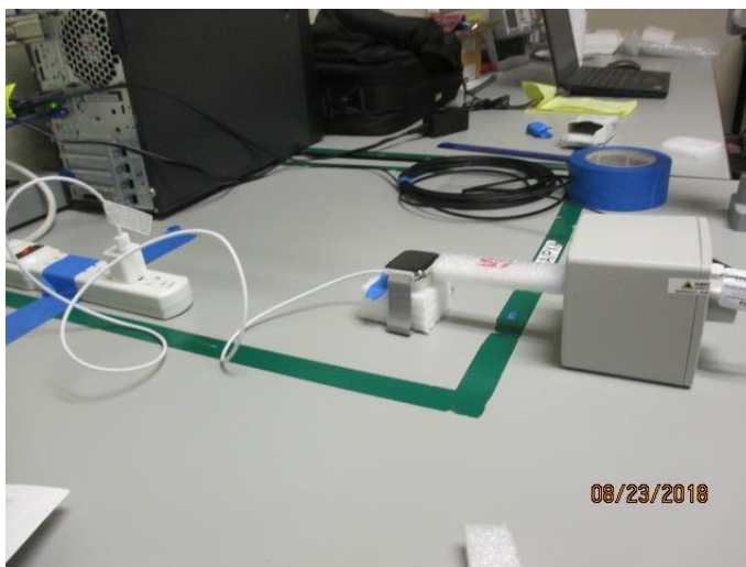
S3, RF EXPOSURE SETUP PHOTO (HORIZONTAL) 15cm
