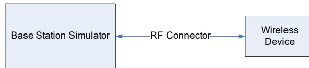
Figure 8-2 Power Measurement Setup
