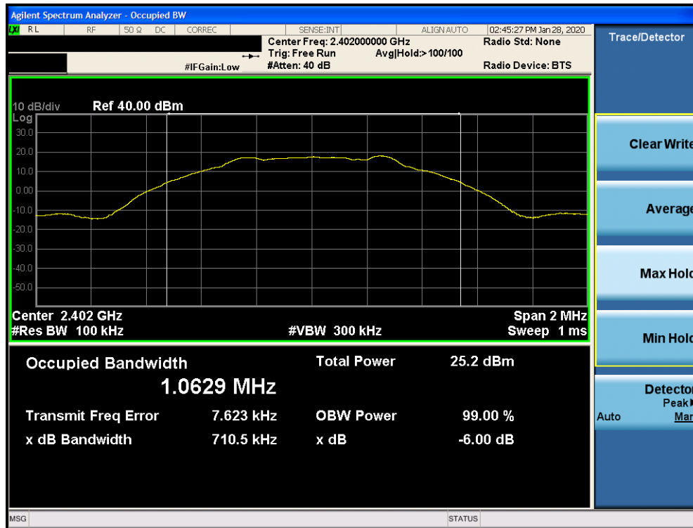
Plot 7-7. 6dB Bandwidth Plot Ant 2a (Bluetooth (LE), 1Mbps, ePA – Ch. 0)
