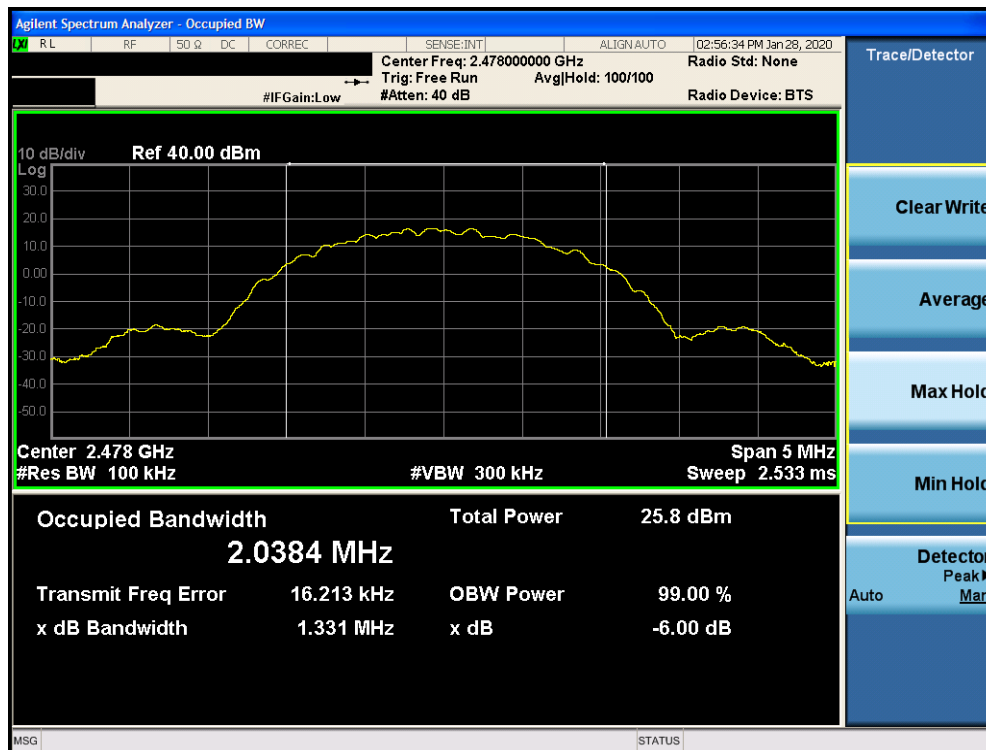
Plot 7-12. 6dB Bandwidth Plot Ant 2a (Bluetooth (LE), 2Mbps, ePA – Ch. 39)
