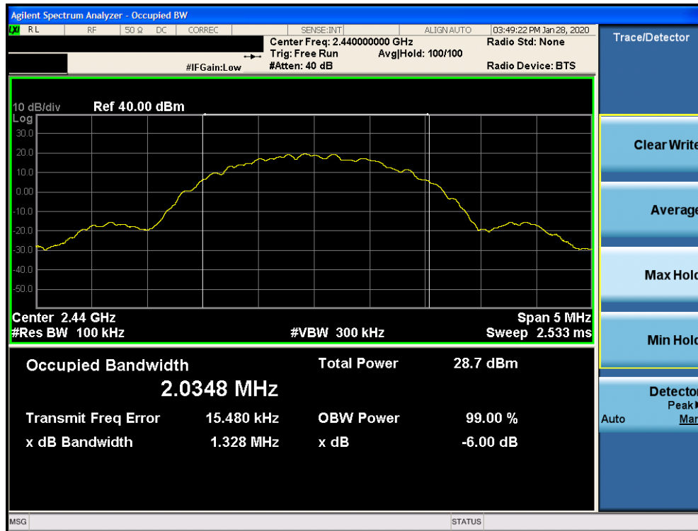
Plot 7-5. 6dB Bandwidth Plot Ant 4a (Bluetooth (LE), 2Mbps, ePA – Ch. 19)
