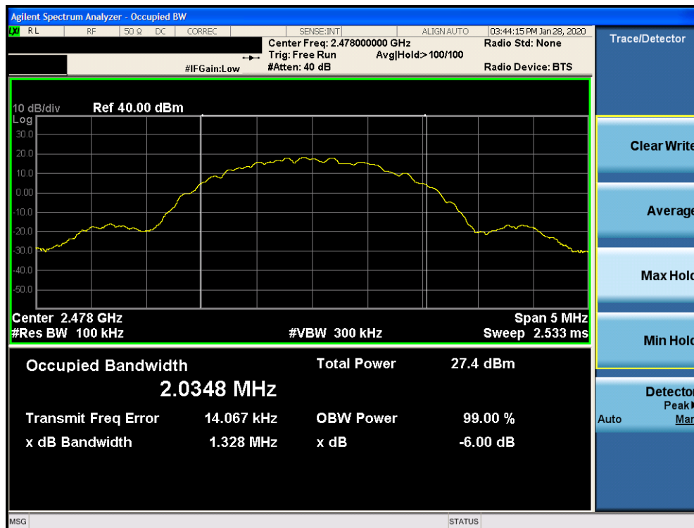
Plot 7-6. 6dB Bandwidth Plot Ant 4a (Bluetooth (LE), 2Mbps, ePA – Ch. 38)
