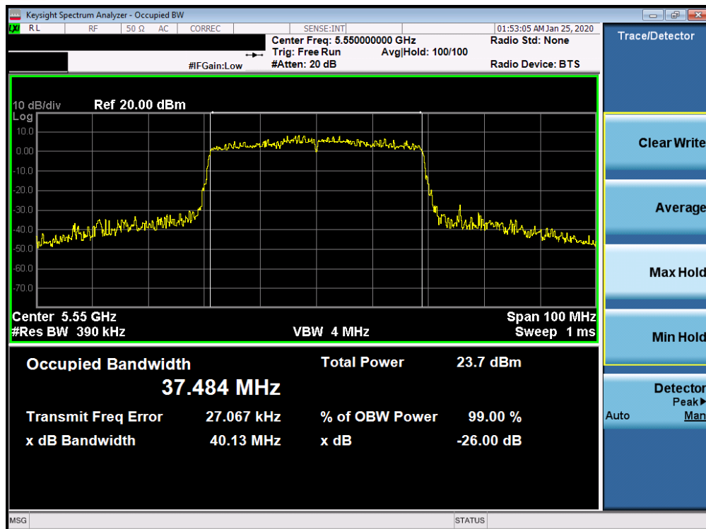
Plot 7-71. 26dB Bandwidth Plot SISO CORE 0 (40MHz BW 802.11ax – RU484 (UNII Band 2C) – Ch. 110)
