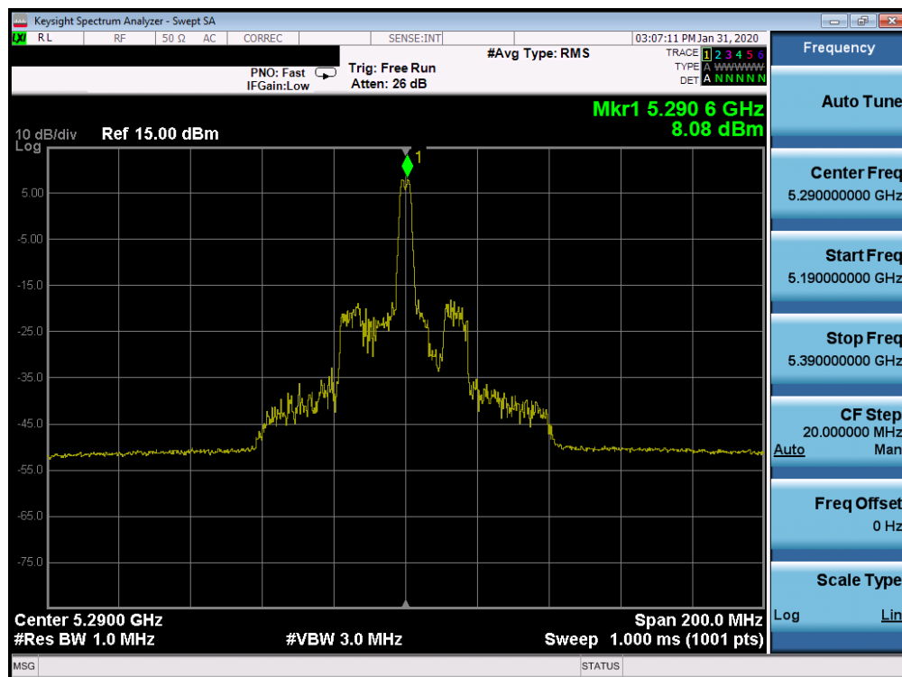
Plot 7-254. Power Spectral Density Plot SISO CORE 0 (80MHz BW 802.11ax Index 18 – RU26 (UNII Band 2A) – Ch. 58)
