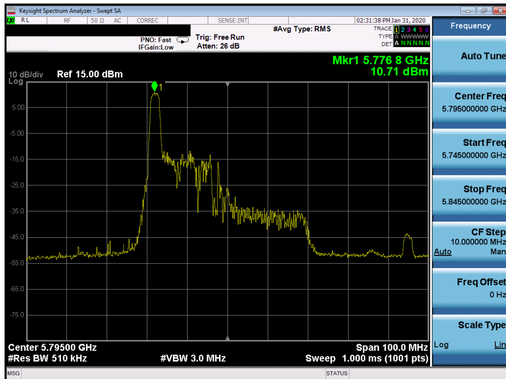
Plot 7-456. Power Spectral Density Plot SISO CORE 1 (40MHz BW 802.11ax Index 0 – RU26 (UNII Band 3) – Ch. 159)
