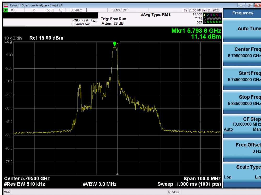
Plot 7-457. Power Spectral Density Plot SISO CORE 1 (40MHz BW 802.11ax Index 8 – RU26 (UNII Band 3) – Ch. 159)
