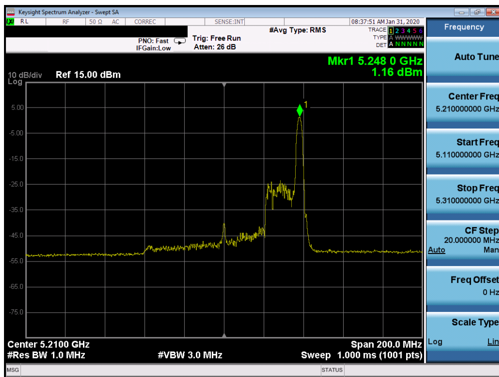
Plot 7-670. Power Spectral Density Plot ISED CDD CORE 1 (80MHz BW 802.11ax Index 36 – RU26 (UNII Band 1) – Ch. 42)
