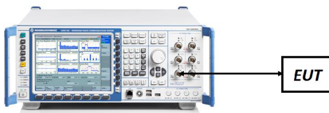
Figure 7-5. ERP/EIRP Measurement Setup
