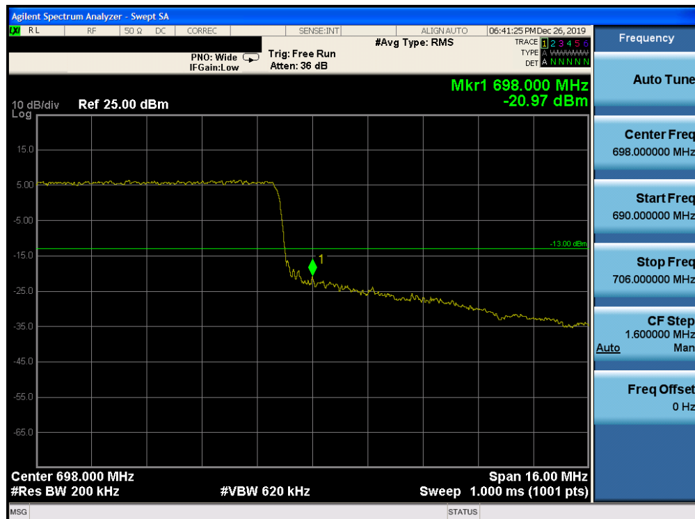
Plot 7-197. Upper Band Edge Plot (Band 71 – 20.0MHz QPSK – RB Size 100)
