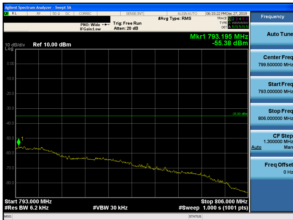
Plot 7-213. Upper Emission Mask Edge Plot (Band 13 – 5.0MHz QPSK – RB Size 25)
