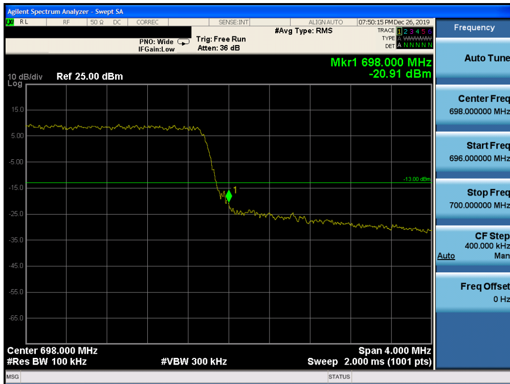
Plot 7-191. Upper Band Edge Plot (Band 71 – 5.0MHz QPSK – RB Size 25)
