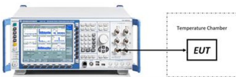
Figure 7-6. Test Instrument & Measurement Setup
