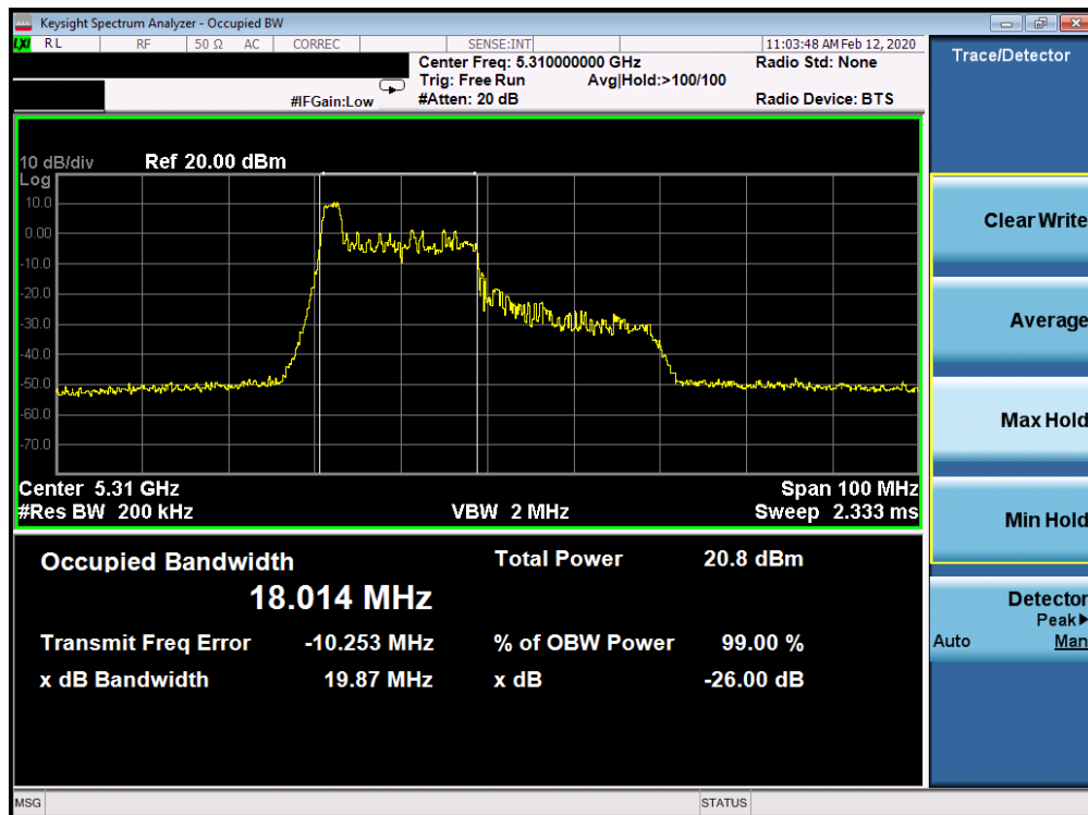
Plot 7-40. 26dB Bandwidth Plot SISO CORE 0 (40MHz BW 802.11ax Index 0 – RU26 (UNII Band 2A) – Ch. 62)
