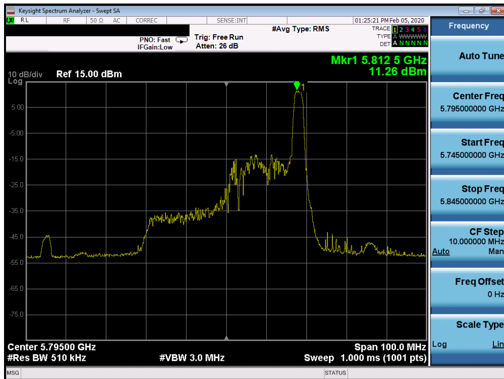
Plot 7-458. Power Spectral Density Plot SISO CORE 1 (40MHz BW 802.11ax Index 17 – RU26 (UNII Band 3) – Ch. 159)
