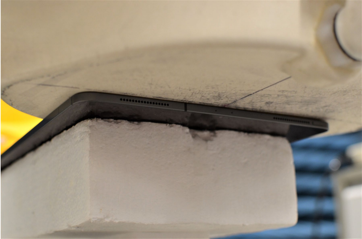
SAR Test Setup Photo 1: Back Side at 0.0 cm – Ant 3/4a/4b
