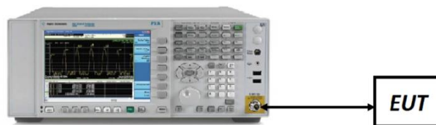
Figure 7-3. Test Instrument & Measurement Setup
