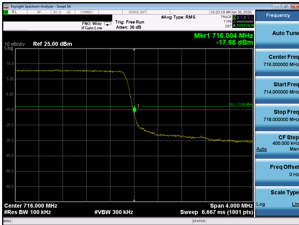
Plot 7-172. Upper Band Edge Plot (Band 12 - 3.0MHz QPSK - Full RB Configuration)
