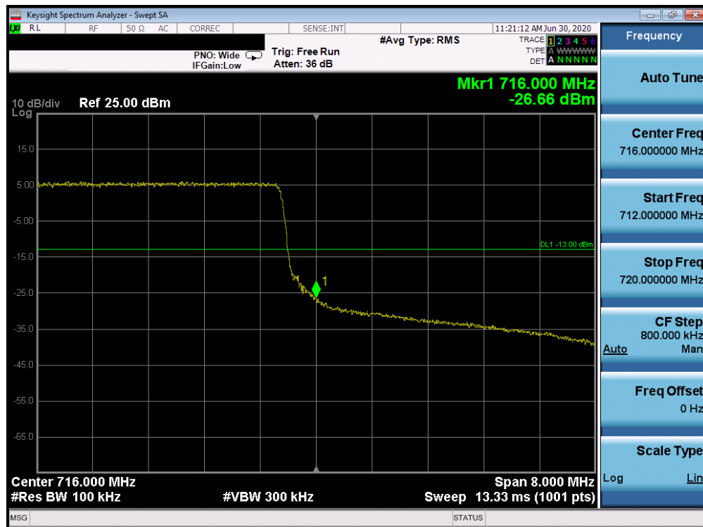
Plot 7-180. Upper Band Edge Plot (Band 17 - 10.0MHz QPSK - Full RB Configuration)
