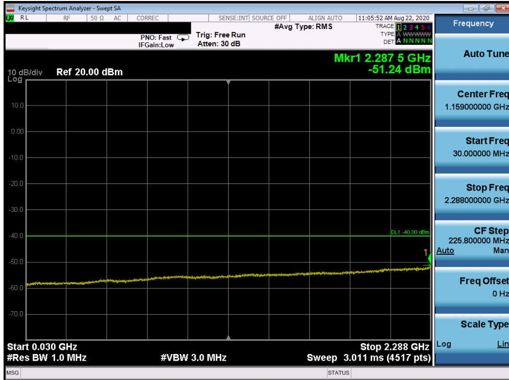
Plot 7-148. Conducted Spurious Plot (Band 30 - 5.0MHz QPSK - RB Size 1, RB Offset 0 - High Channel)
