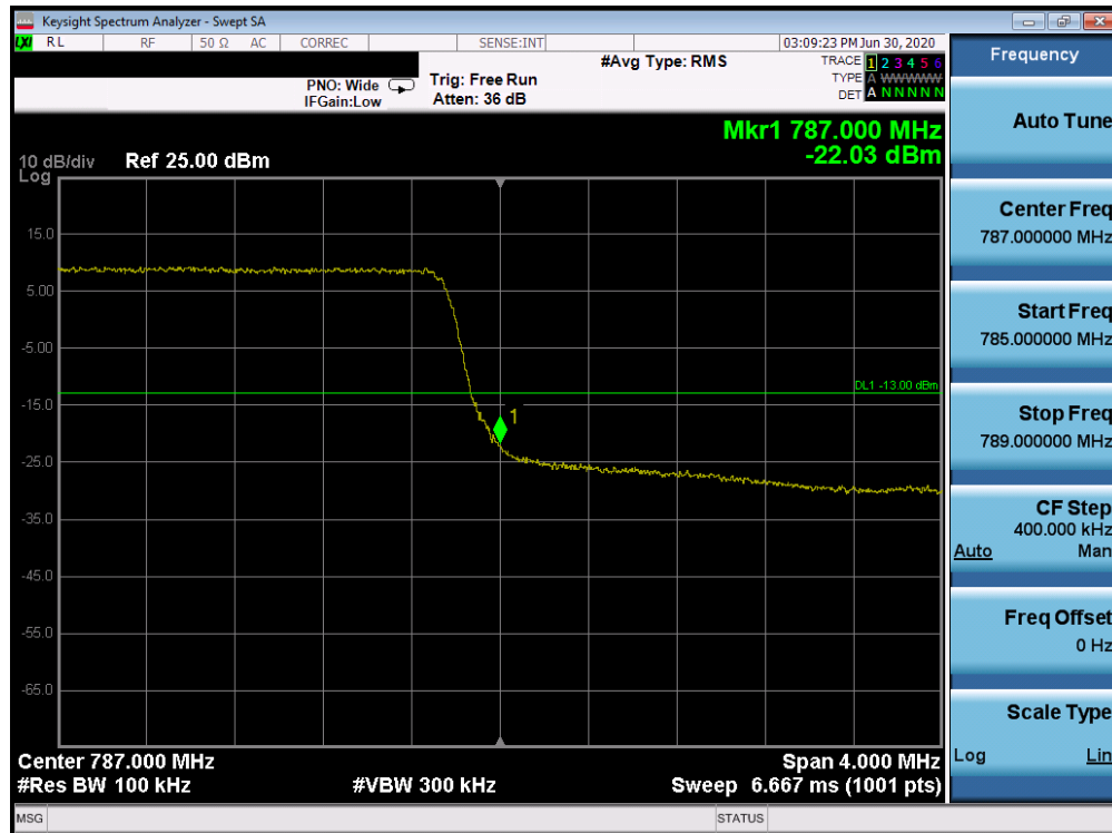
Plot 7-183. Upper Band Edge Plot (Band 13 - 5.0MHz QPSK - Full RB Configuration)
