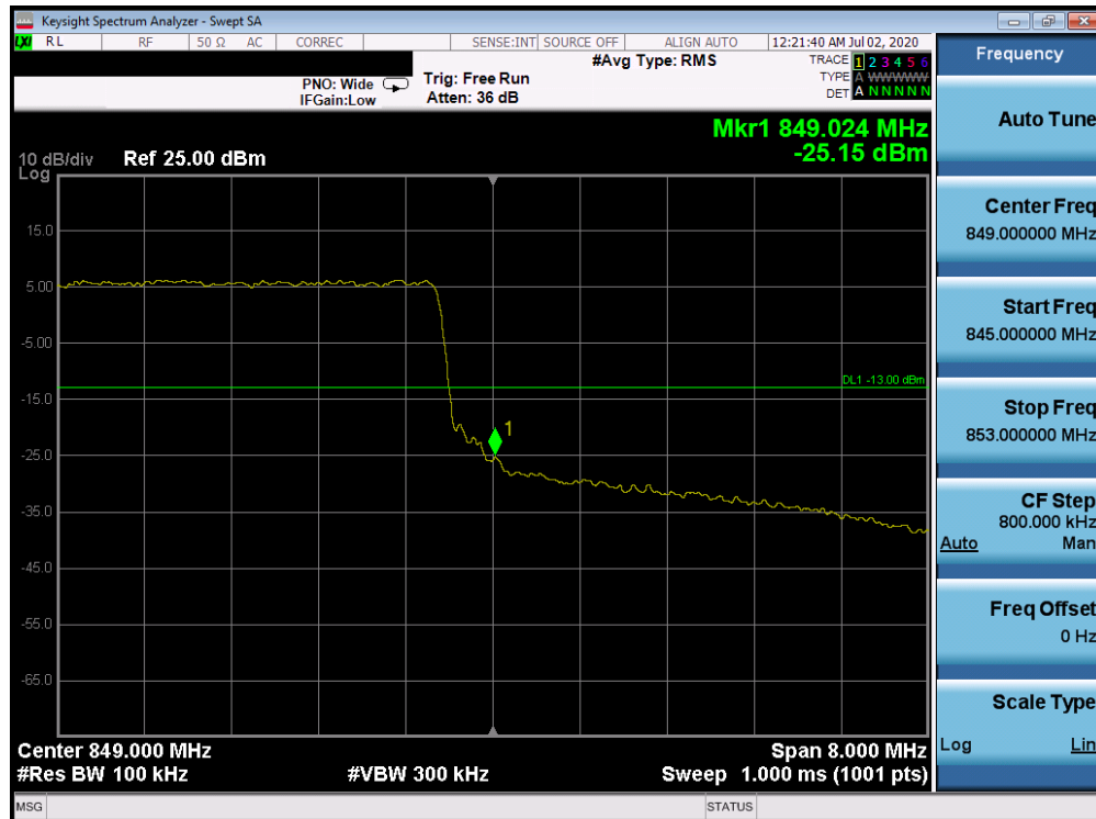
Plot 7-196. Upper Band Edge Plot (Band 26 - 10.0MHz QPSK - Full RB Configuration)
