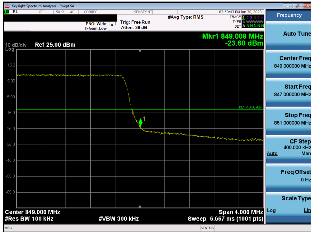
Plot 7-202. Upper Band Edge Plot (Band 5 - 5.0MHz QPSK - Full RB Configuration)
