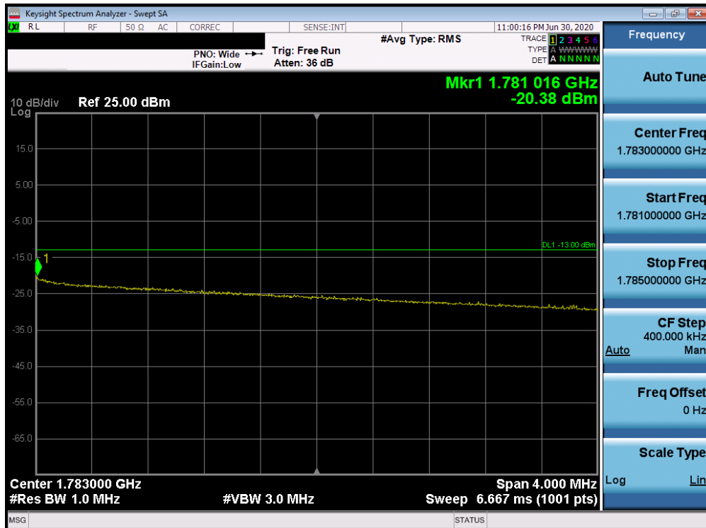
Plot 7-220. Upper Extended Band Edge Plot (Band 66 - 10.0MHz QPSK - Full RB Configuration)
