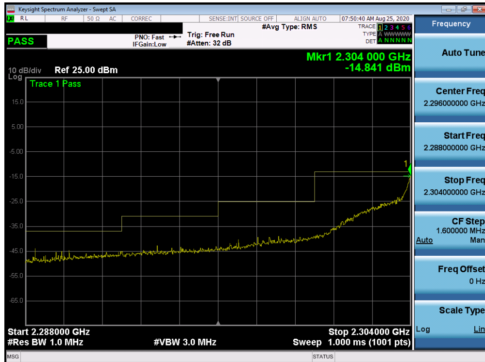
Plot 7-302. Lower Extended Band Edge Plot (Band 30 - 5.0MHz QPSK - Full RB Configuration)
