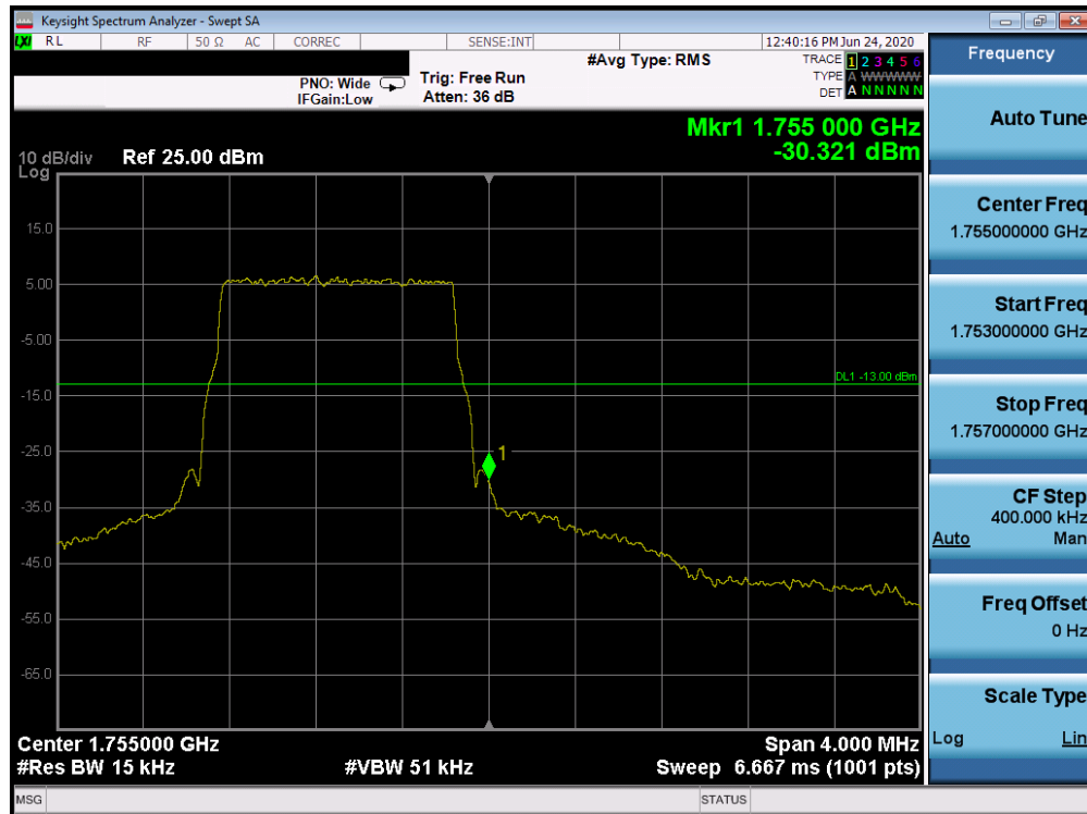
Plot 7-231. Upper Band Edge Plot (Band 4 - 1.4MHz QPSK - Full RB Configuration)
