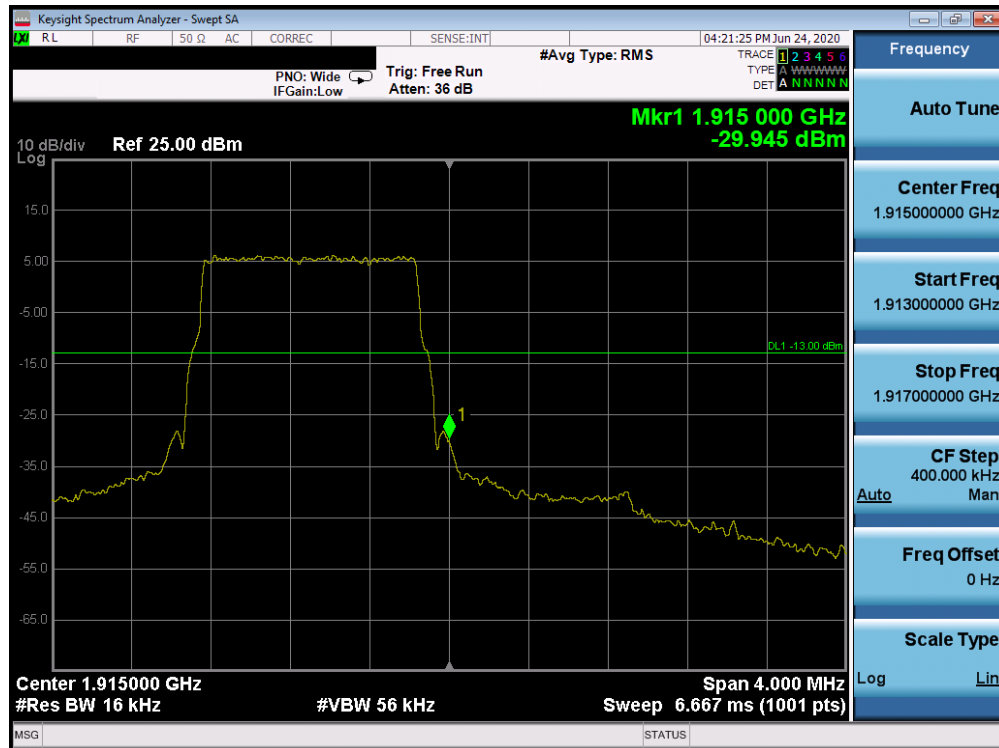
Plot 7-255. Upper Band Edge Plot (Band 25 - 1.4MHz QPSK - Full RB Configuration)
