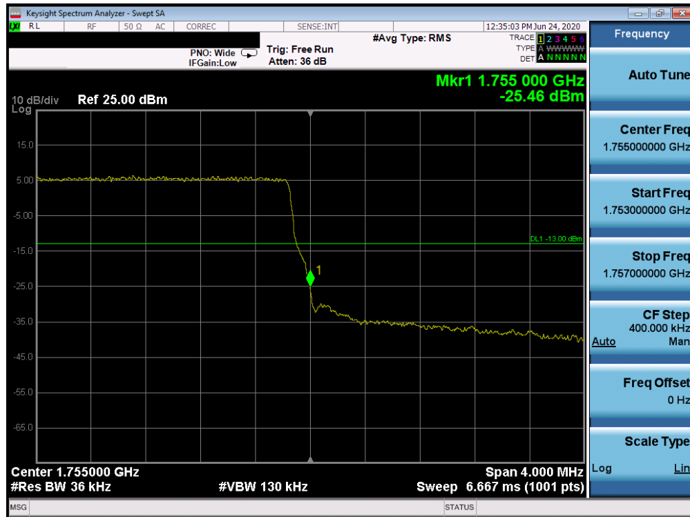
Plot 7-235. Upper Band Edge Plot (Band 4 - 3.0MHz QPSK - Full RB Configuration)
