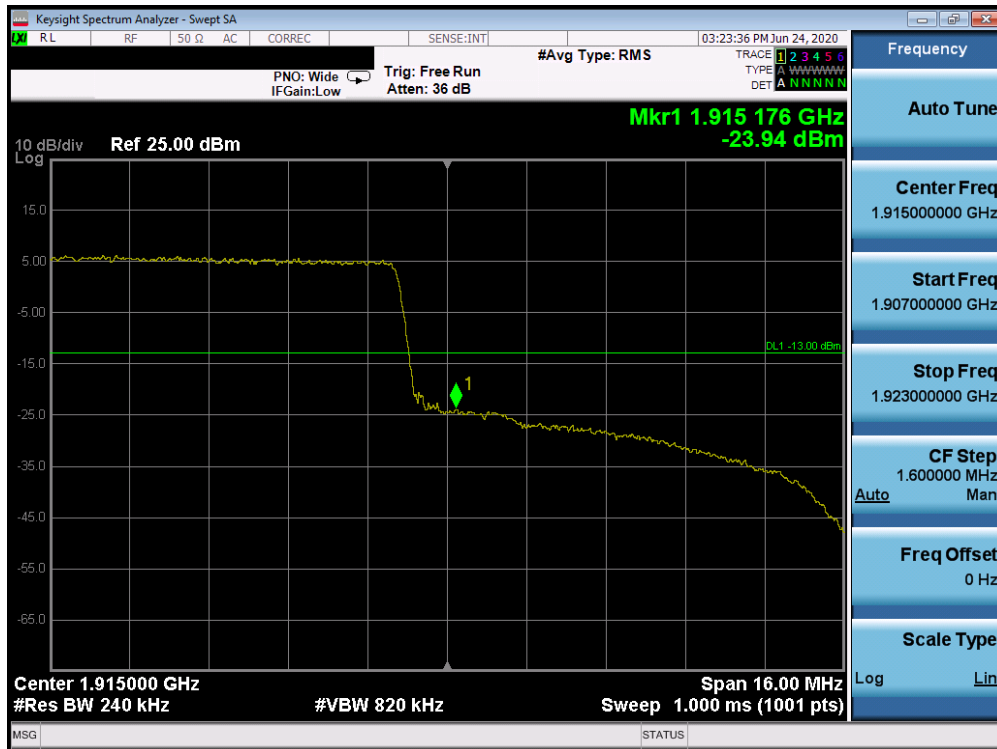
Plot 7-275. Upper Band Edge Plot (Band 25 - 20.0MHz QPSK - Full RB Configuration)
