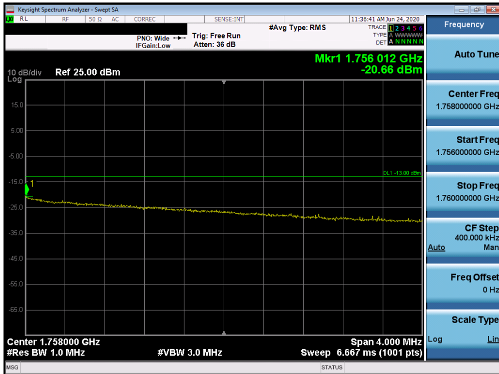
Plot 7-244. Upper Extended Band Edge Plot (Band 4 - 10.0MHz QPSK - Full RB Configuration)
