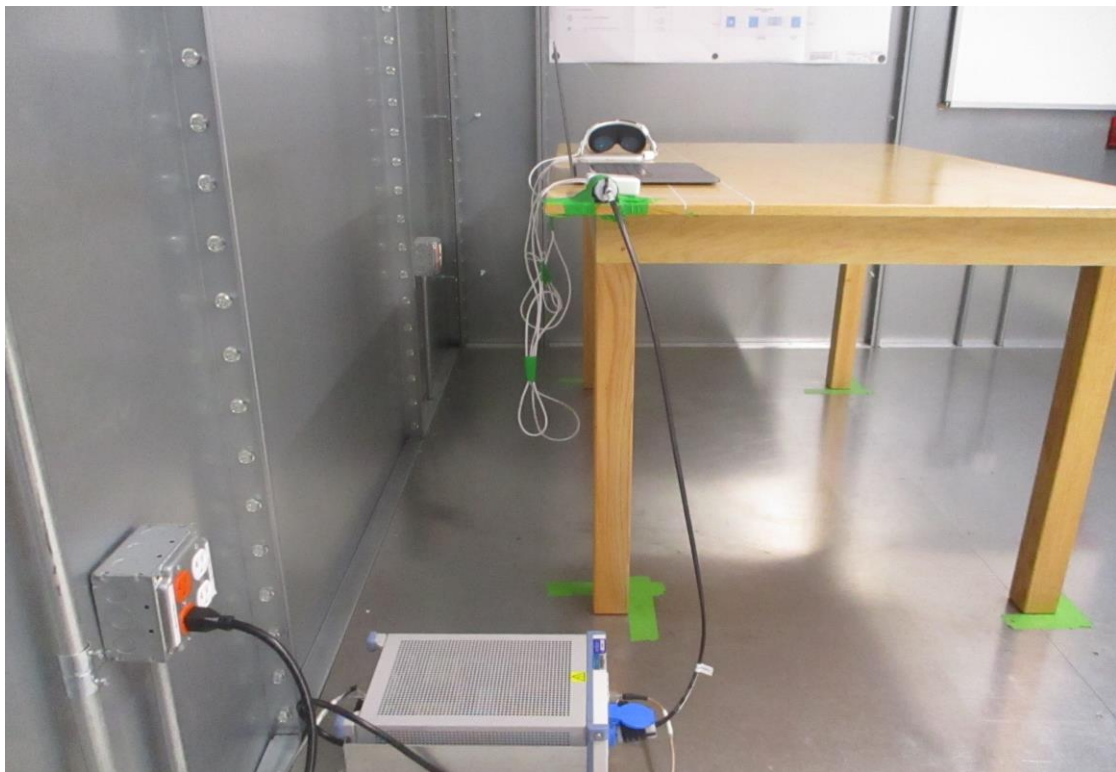
Figure 4: AC Line Conducted Emissions (Side View)
