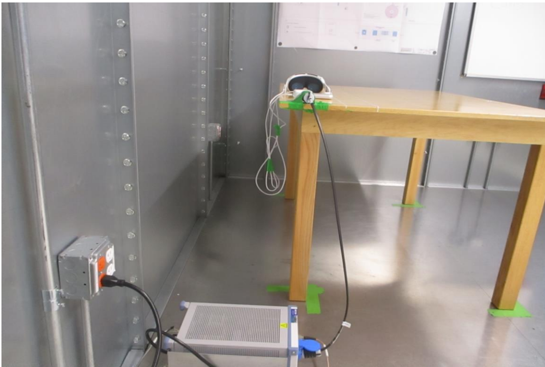
Figure 2: AC Line Conducted Emissions (Side View)
