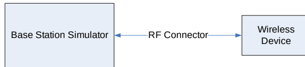
Figure 8-2 Power Measurement Setup
