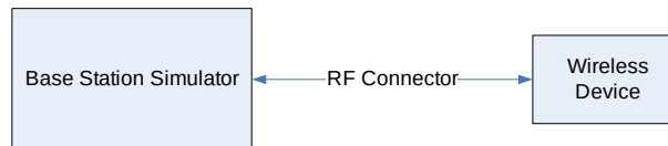
Figure 8-3 Power Measurement Setup
