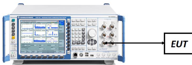
Figure 7-5. ERP/EIRP Measurement Setup
