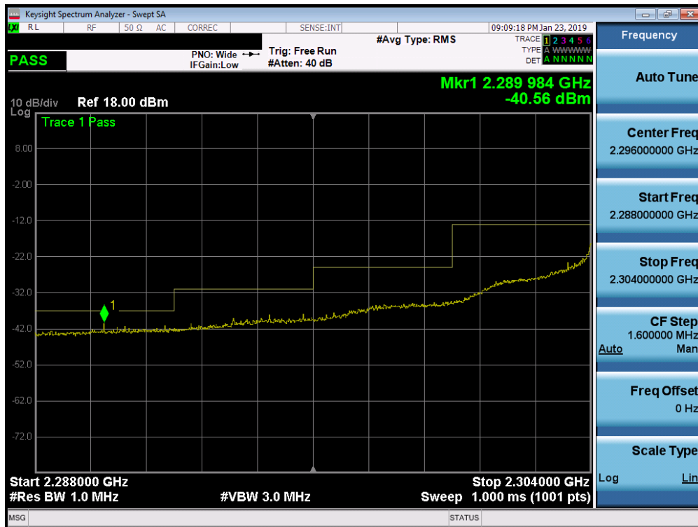
Plot 7-298. Lower Extended Band Edge Plot (Band 30 - 5.0MHz QPSK - Full RB Configuration)
