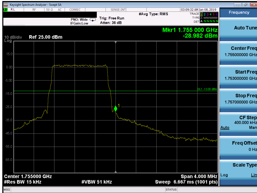
Plot 7-227. Upper Band Edge Plot (Band 4 - 1.4MHz QPSK - Full RB Configuration)
