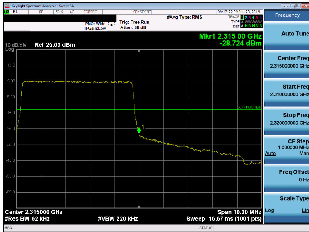
Plot 7-299. Upper Band Edge Plot (Band 30 - 5.0MHz QPSK - Full RB Configuration)
