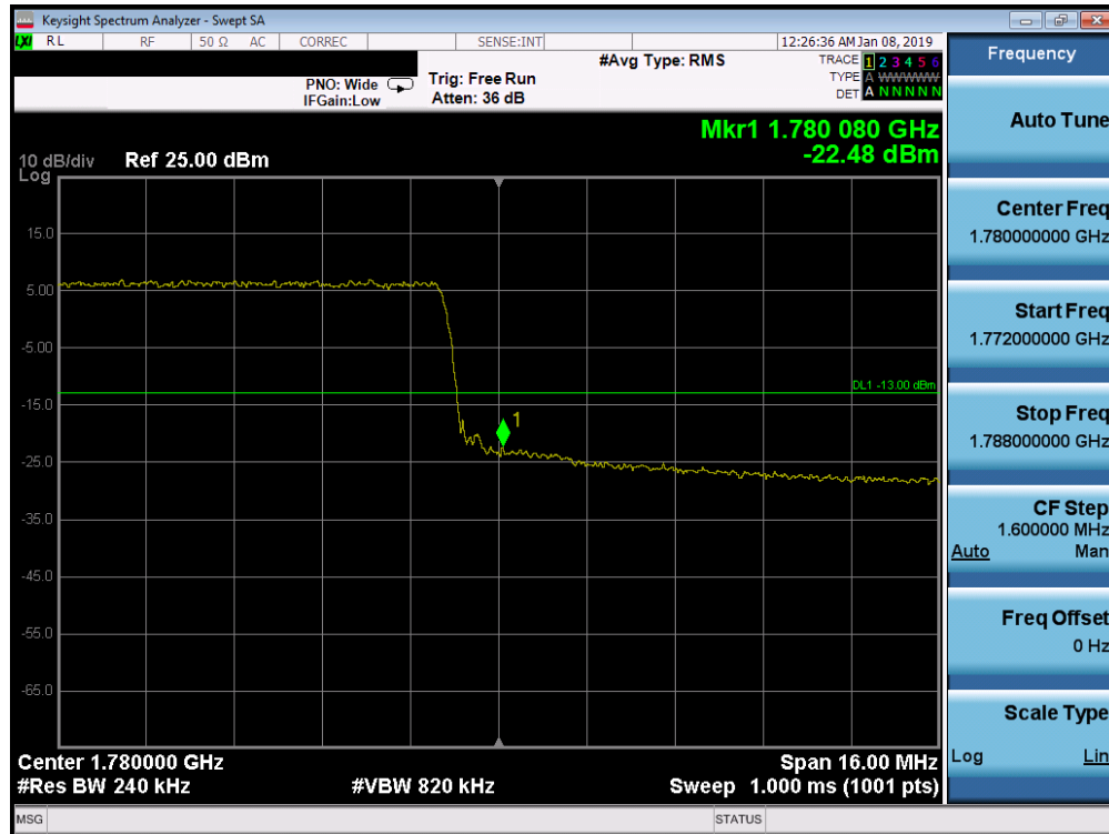
Plot 7-223. Upper Band Edge Plot (Band 66 - 20.0MHz QPSK - Full RB Configuration)
