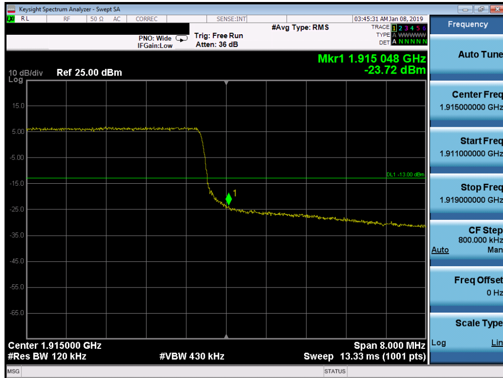
Plot 7-263. Upper Band Edge Plot (Band 25 - 10.0MHz QPSK - Full RB Configuration)
