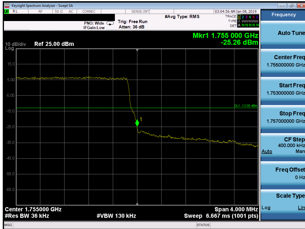
Plot 7-231. Upper Band Edge Plot (Band 4 - 3.0MHz QPSK - Full RB Configuration)
