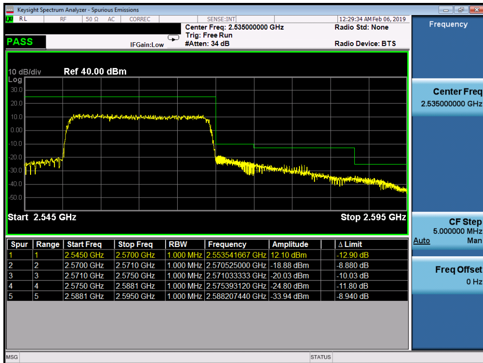
Plot 7-312. Upper ACP Plot (Band 7 - 20.0MHz QPSK - Full RB Configuration)
