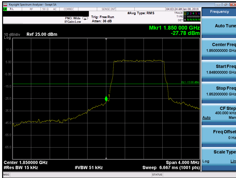
Plot 7-273. Lower Band Edge Plot (Band 2 - 1.4MHz QPSK - Full RB Configuration)
