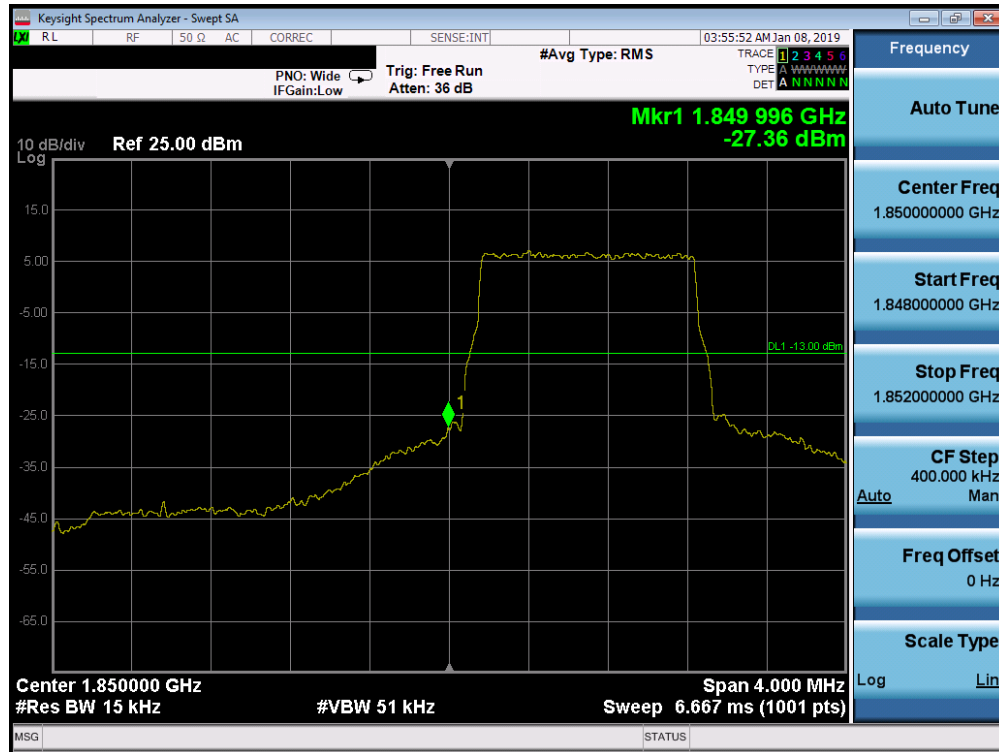
Plot 7-249. Lower Band Edge Plot (Band 25 - 1.4MHz QPSK - Full RB Configuration)
