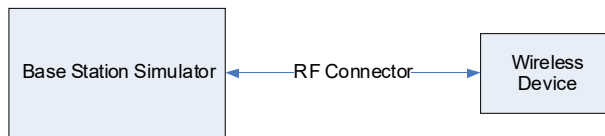
Figure 8-2 Power Measurement Setup
