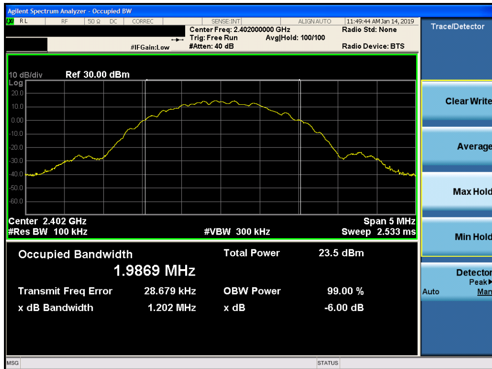
Plot 7-16. 6dB Bandwidth Plot ANT 2 (Bluetooth (LE), 2Mbps ePA – Ch. 0)
