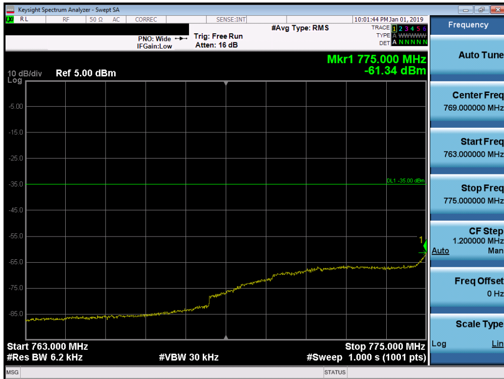
Plot 7-186. Lower Emission Mask Edge Plot (Band 13 - 10.0MHz QPSK - Full RB Configuration)
