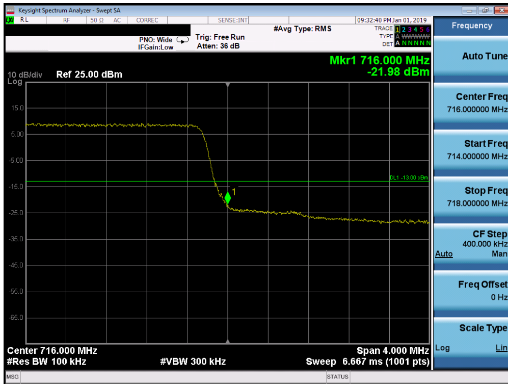
Plot 7-178. Higher Band Edge Plot (Band 17 - 5.0MHz QPSK - Full RB Configuration)
