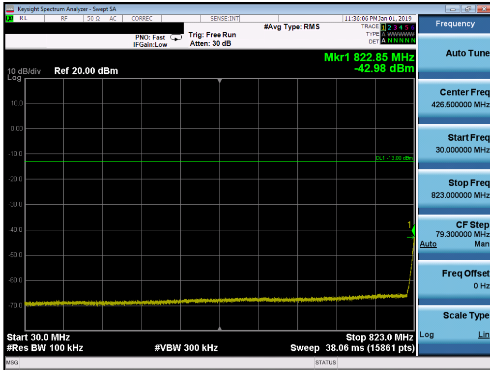
Plot 7-115. Conducted Spurious Plot (Band 26/5 - 10.0MHz QPSK - RB Size 1, RB Offset 0 - Low Channel)
