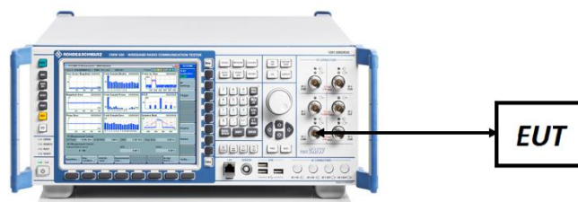
Figure 7-4. Conducted Power Measurement Setup
