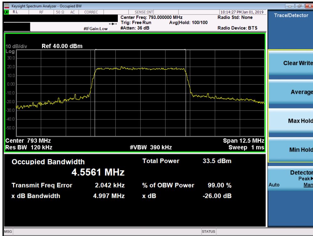
Plot 7-14. Occupied Bandwidth Plot (LTE Band 14, 5MHz 16-QAM – RB Size 25)
