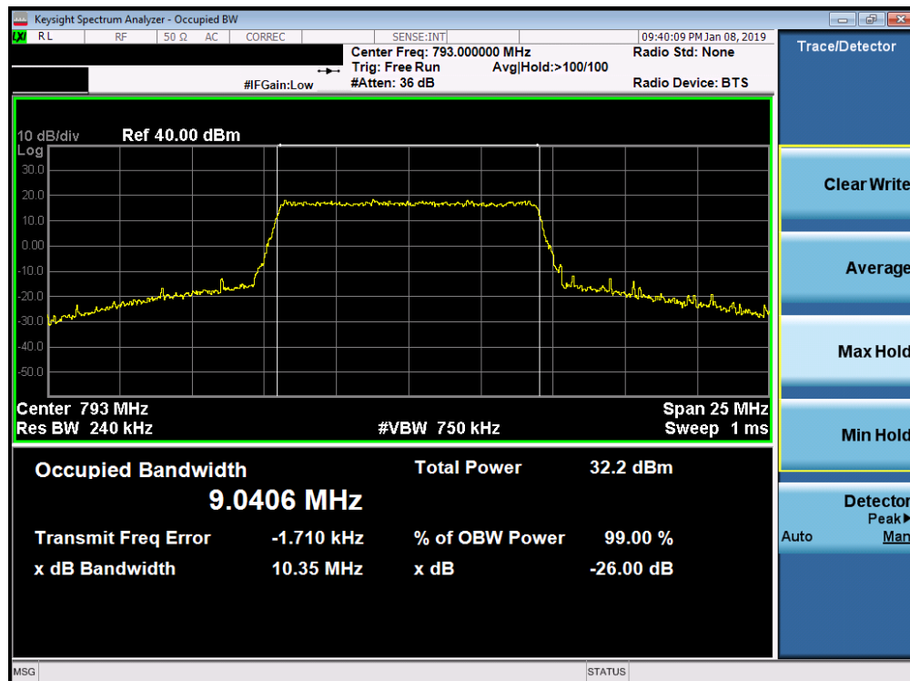
Plot 7-18. Occupied Bandwidth Plot (LTE Band 14, 10MHz 64-QAM – RB Size 50)
