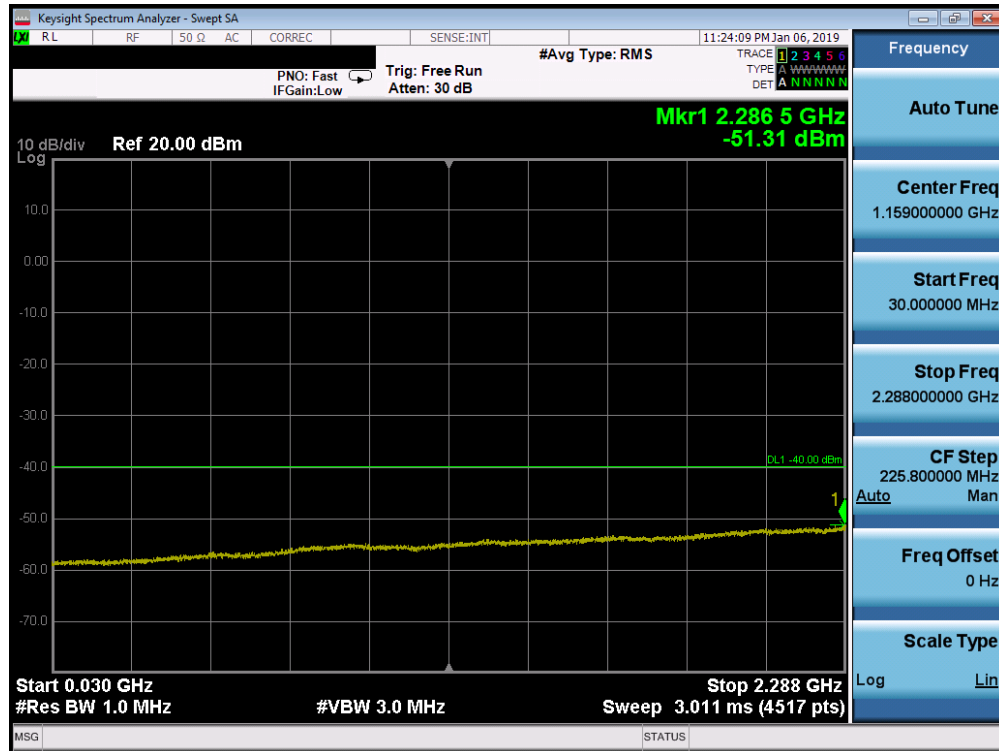
Plot 7-169. Conducted Spurious Plot (Band 30 - 5.0MHz QPSK - RB Size 1, RB Offset 0 - High Channel)
