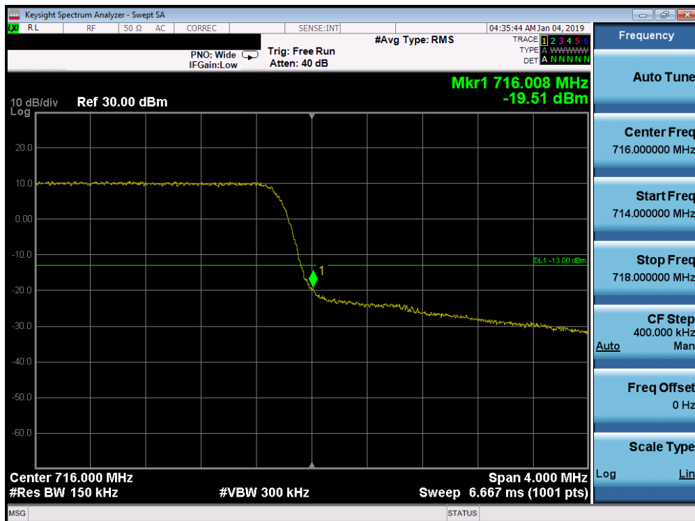
Plot 7-203. Upper Band Edge Plot (Band 12 - 5.0MHz QPSK - Full RB Configuration)
