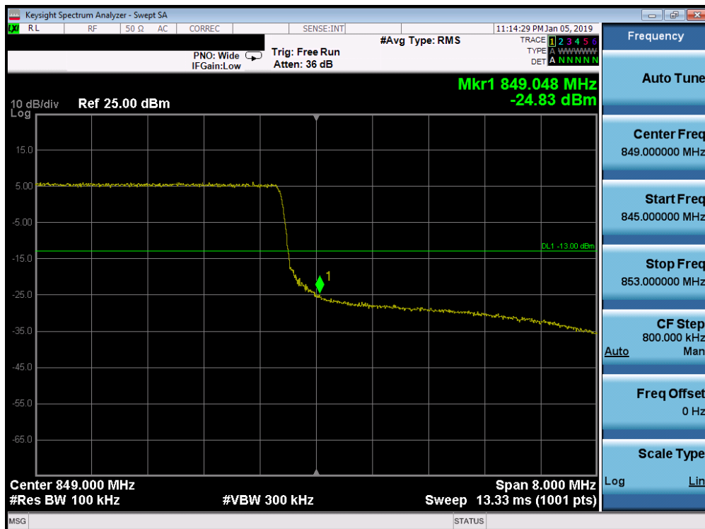
Plot 7-225. Upper Band Edge Plot (Band 5 - 10.0MHz QPSK - Full RB Configuration)
