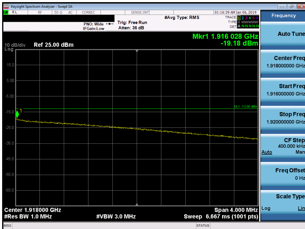
Plot 7-321. Upper Extended Band Edge Plot (Band 25 - 10.0MHz QPSK - Full RB Configuration)
