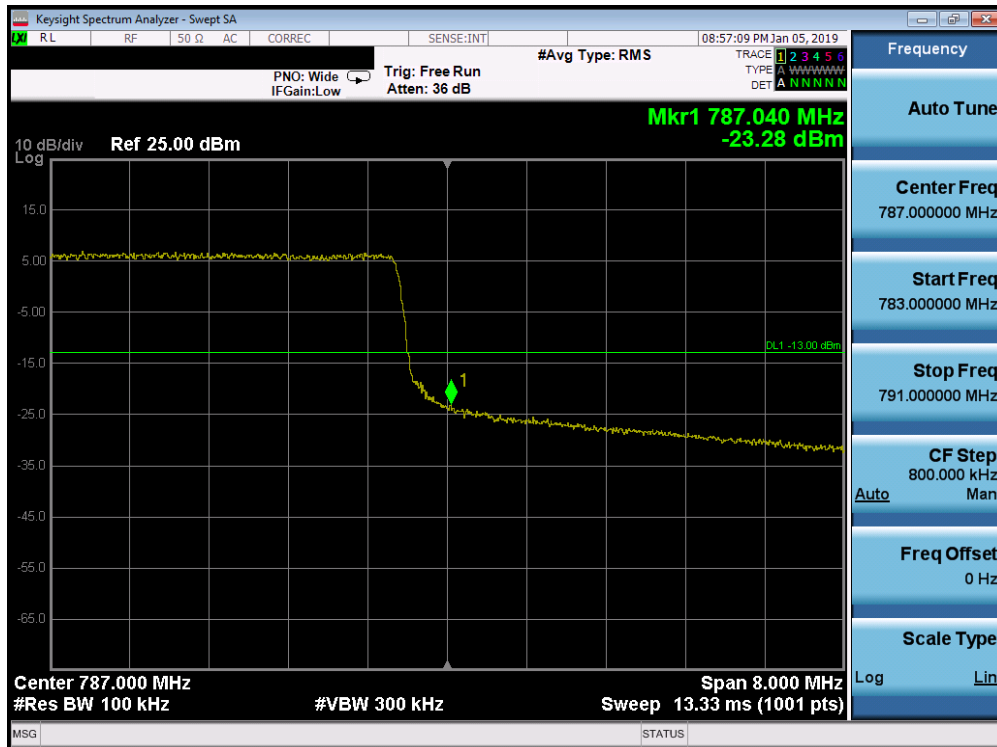
Plot 7-216. Upper Band Edge Plot (Band 13 - 10.0MHz QPSK - Full RB Configuration)
