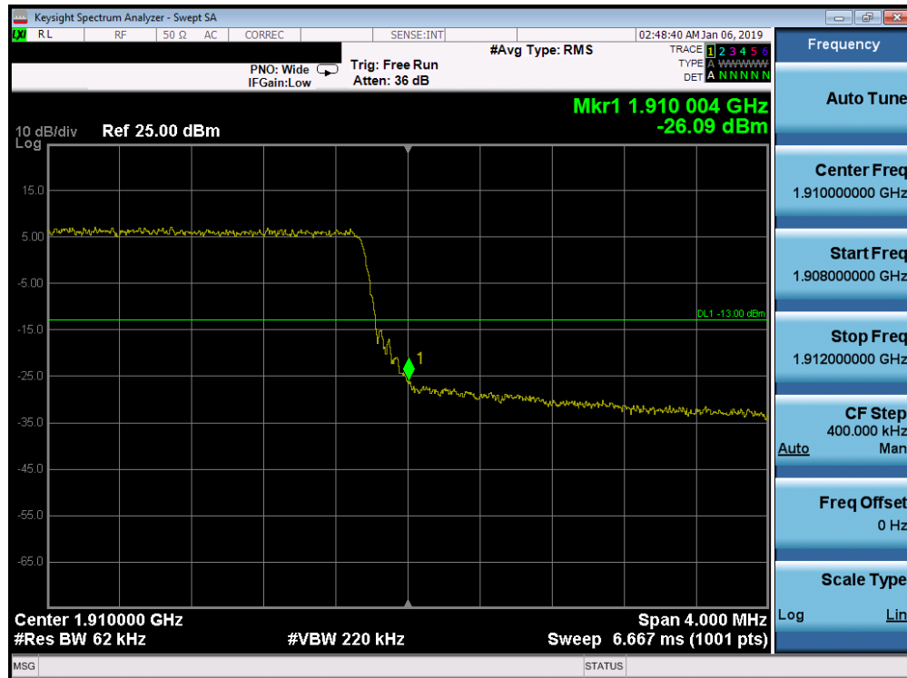
Plot 7-292. Upper Band Edge Plot (Band 2 - 5.0MHz QPSK - Full RB Configuration)
