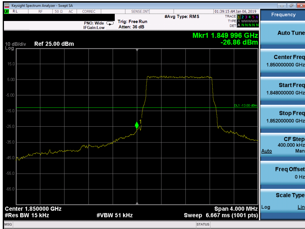
Plot 7-306. Lower Band Edge Plot (Band 25 - 1.4MHz QPSK - Full RB Configuration)
