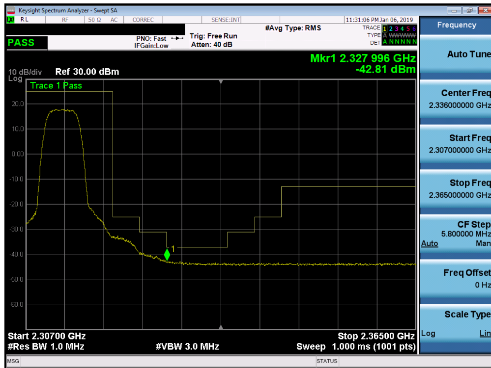
Plot 7-333. Upper Extended Band Edge Plot (Band 30 - 5.0MHz QPSK - Full RB Configuration)
