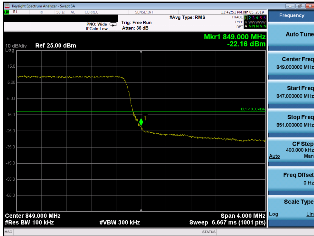
Plot 7-231. Upper Band Edge Plot (Band 26 - 5.0MHz QPSK - Full RB Configuration)
