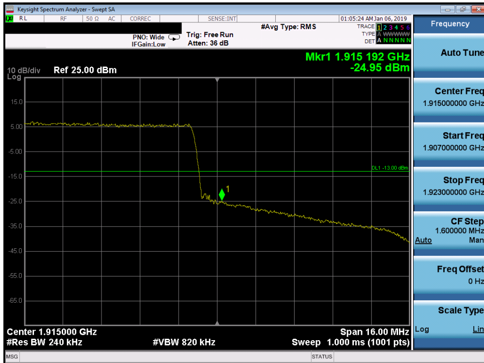
Plot 7-328. Upper Band Edge Plot (Band 25 - 20.0MHz QPSK - Full RB Configuration)
