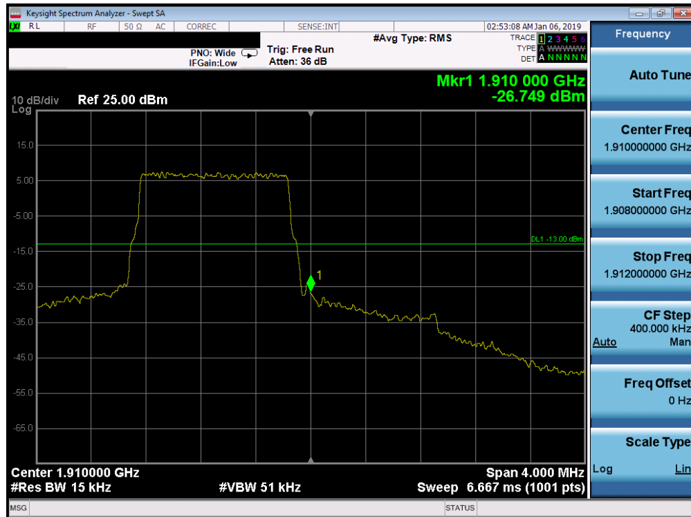
Plot 7-284. Upper Band Edge Plot (Band 2 - 1.4MHz QPSK - Full RB Configuration)
