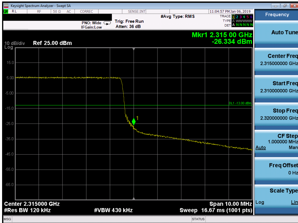
Plot 7-336. Upper Band Edge Plot (Band 30 - 10.0MHz QPSK - Full RB Configuration)
