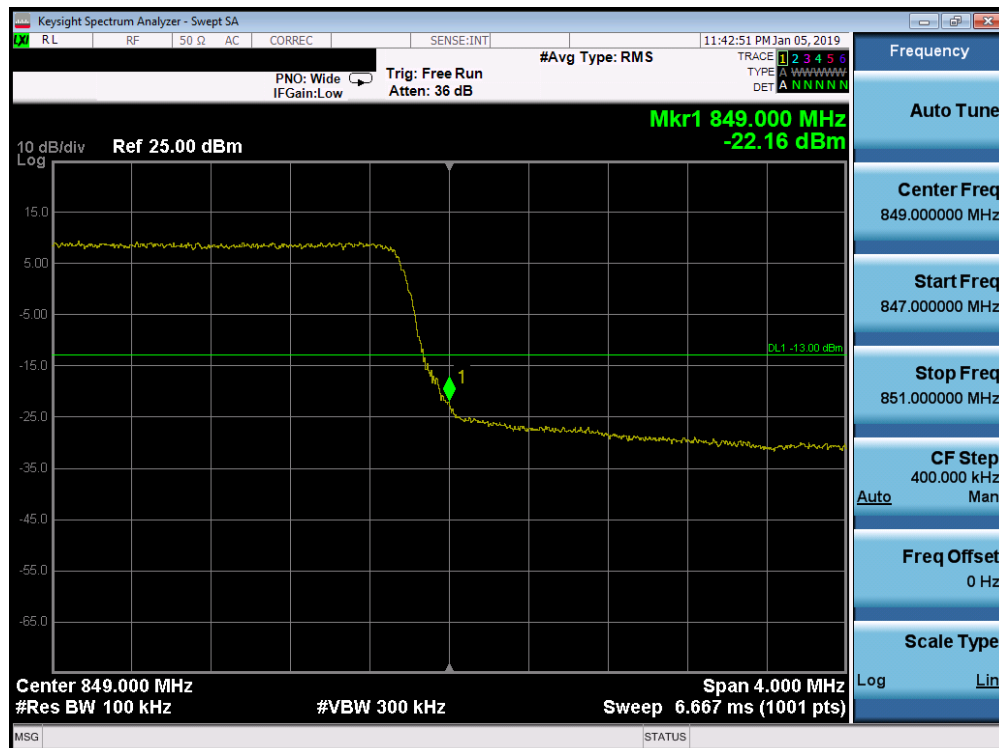
Plot 7-223. Upper Band Edge Plot (Band 5 - 5.0MHz QPSK - Full RB Configuration)
