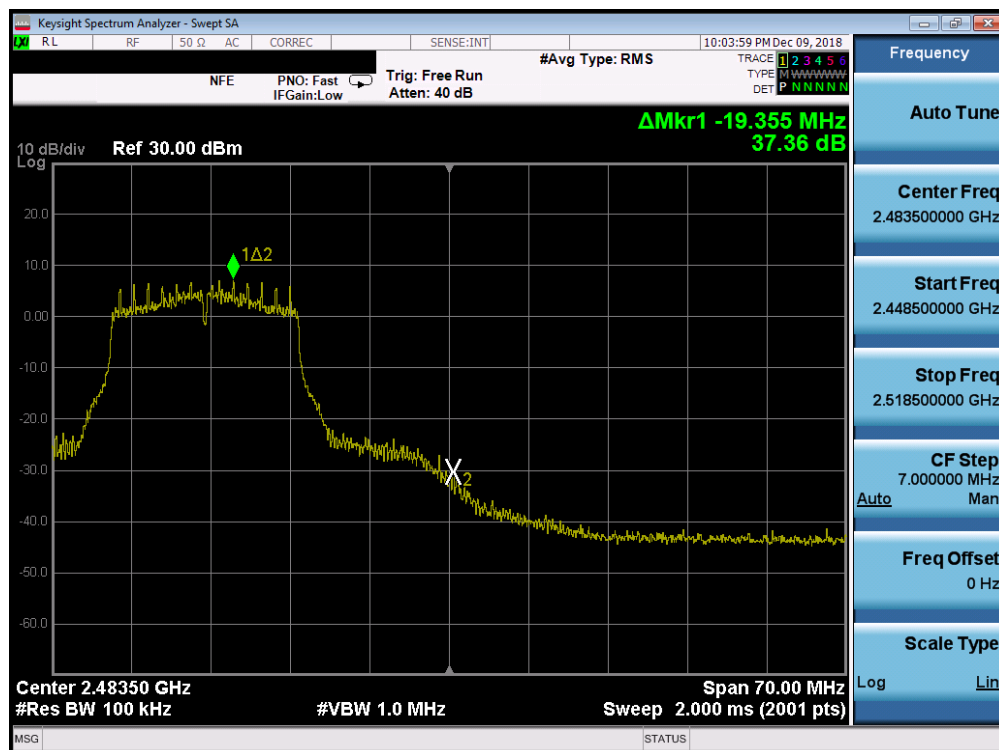
Plot 7-54. Band Edge Plot SISO CORE 0 (802.11g - Ch. 11)
