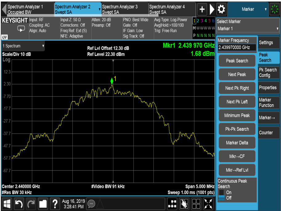
Figure 7 - 2440 MHz, Power Spectral Density
