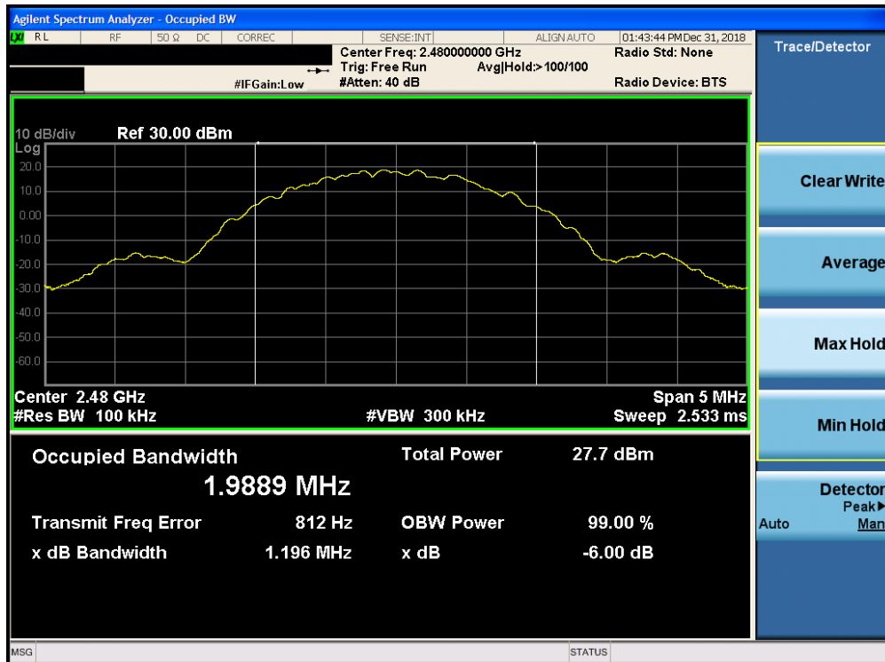
Plot 7-12. 6dB Bandwidth Plot ANT 1 (Bluetooth (LE), 2Mbps ePA – Ch. 39)
