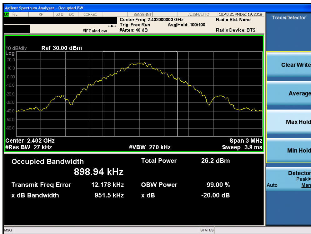
Plot 7-1. 20dB Bandwidth Plot ANT 0 (Bluetooth, GFSK, ePA – Ch. 0)
