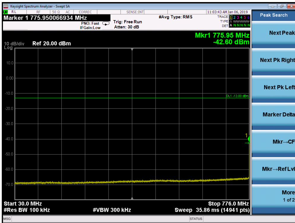
Plot 7-139. Conducted Spurious Plot (Band 26/5 - 10.0MHz QPSK - RB Size 1, RB Offset 0 - Mid Channel)
