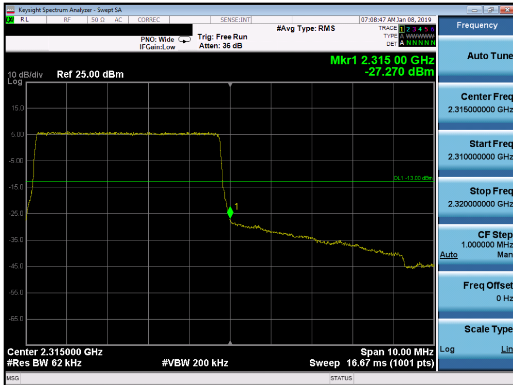
Plot 7-328. Upper Band Edge Plot (Band 30 - 5.0MHz QPSK - Full RB Configuration)
