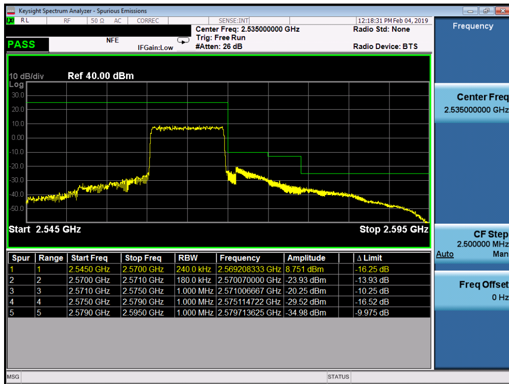
Plot 7-337. Upper ACP Plot (Band 7 - 10.0MHz QPSK - Full RB Configuration)
