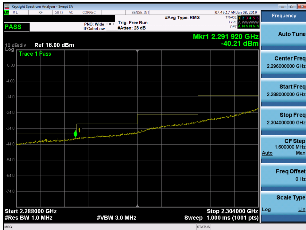
Plot 7-331. Lower Extended Band Edge Plot (Band 30 - 10.0MHz QPSK - Full RB Configuration)
