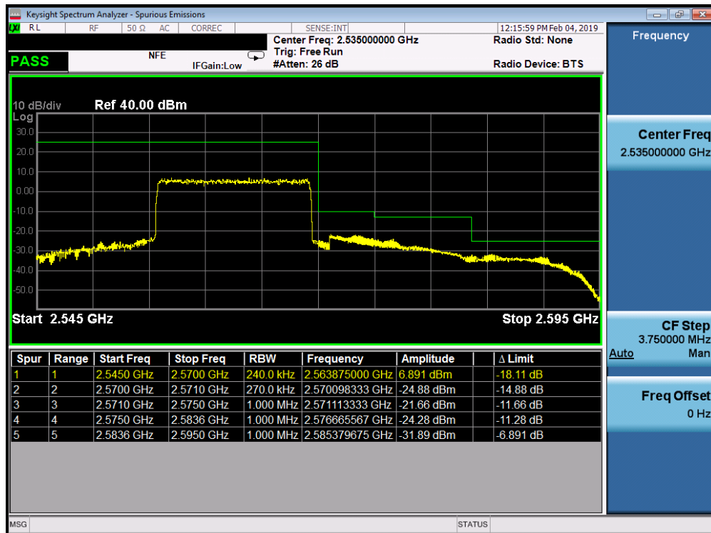
Plot 7-339. Upper ACP Plot (Band 7 - 15.0MHz QPSK - Full RB Configuration)
