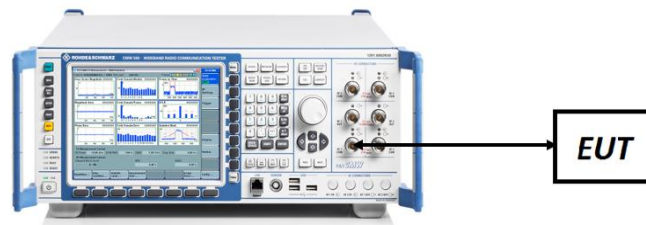
Figure 7-5. Conducted Power Measurement Setup
