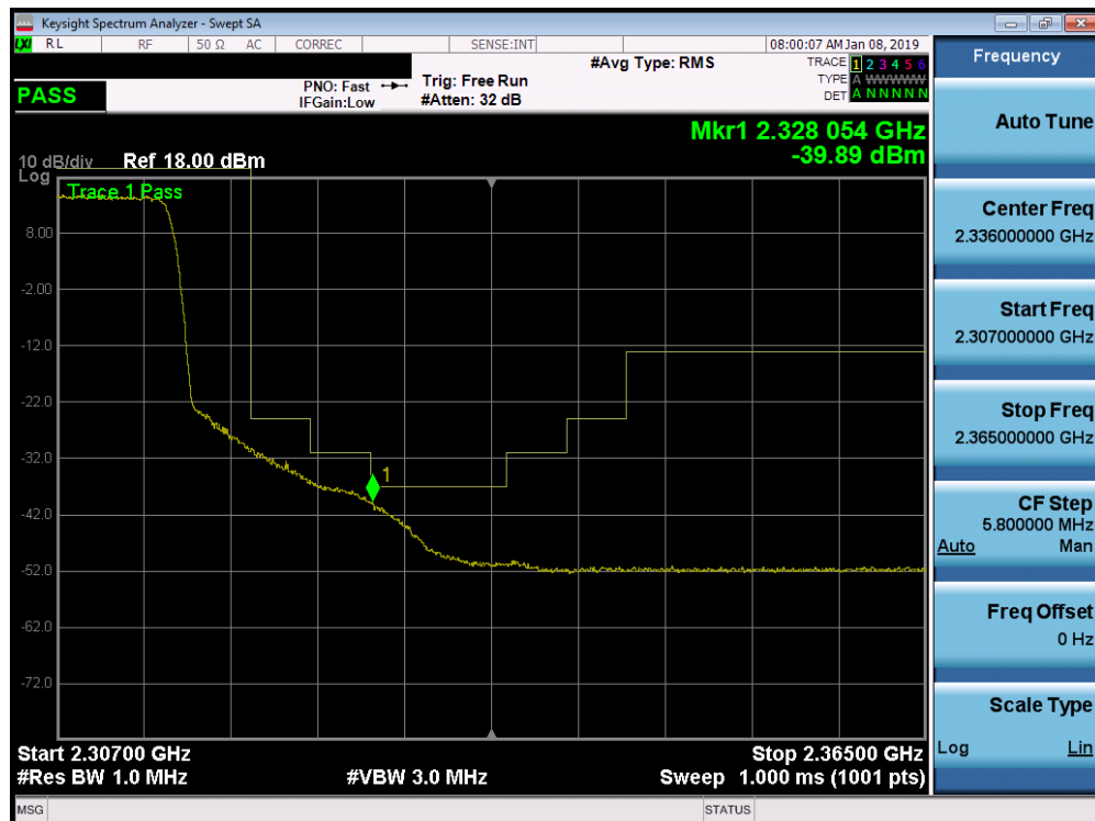
Plot 7-333. Upper Extended Band Edge Plot (Band 30 - 10.0MHz QPSK - Full RB Configuration)
