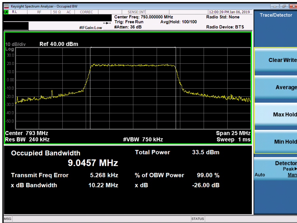
Plot 7-16. Occupied Bandwidth Plot (LTE Band 14, 10MHz QPSK – RB Size 50)
