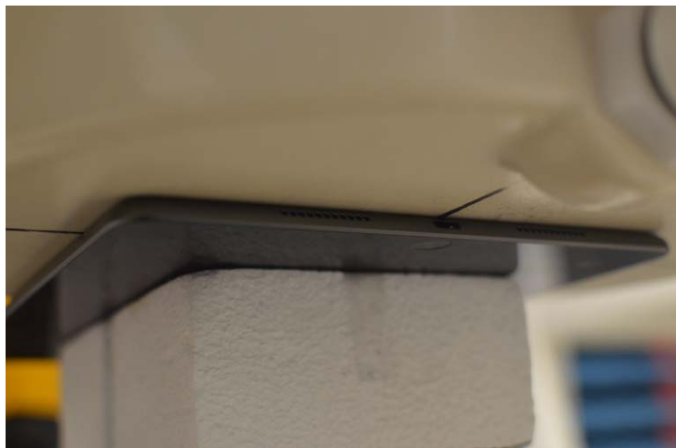
SAR Test Setup Photo 2: Back Side at 0.0 cm – ANTWF1/WF2
