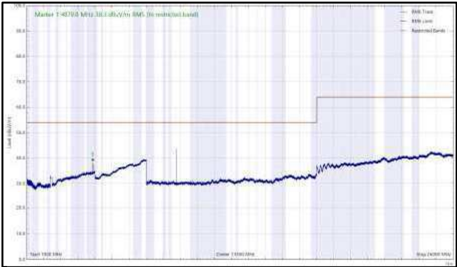
Figure 277 - 2440 MHz (CH17), LE1M, ePA, Core 1, 1 GHz to 26 GHz, Vertical (RMS)
