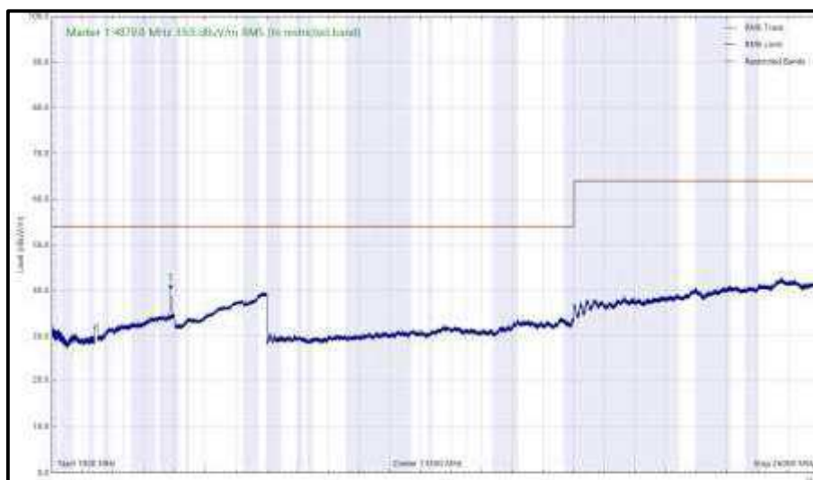
Figure 319 - 2440 MHz (CH17), LE1M, iPA, Core 2, 1 GHz to 26 GHz, Vertical (RMS)
