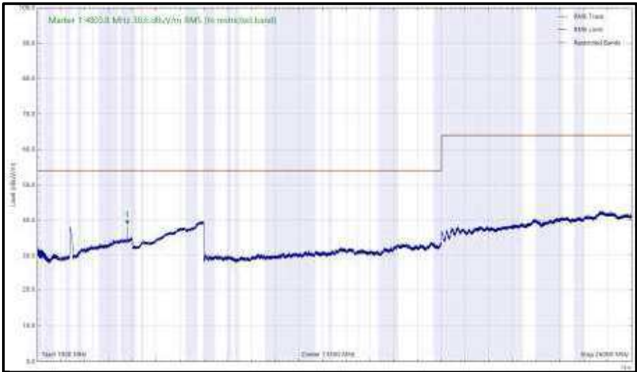
Figure 299 - 2402 MHz (CH0), LE1M, iPA, Core 1, 1 GHz to 26 GHz, Vertical (RMS)
