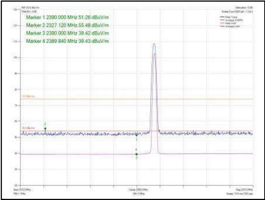
Figure 241 – Static - Core 2 - GFSK/DH1 - 2402 MHz - Band Edge Frequency 2390.0 MHz
